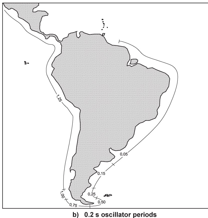
Figure B.4—5 % Damped Spectral Response Accelerations for Offshore South America (Continued)
