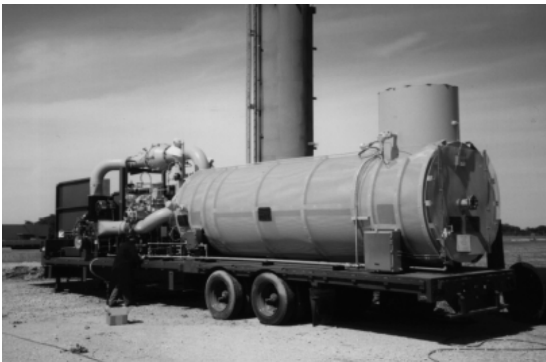
Figure 5-3—Example of Tank Mechanical Vapor-Freeing Equipment
