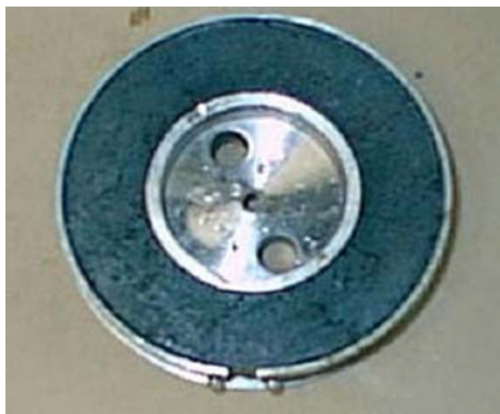
Figure 1 — Typical mould assembly (top view)
