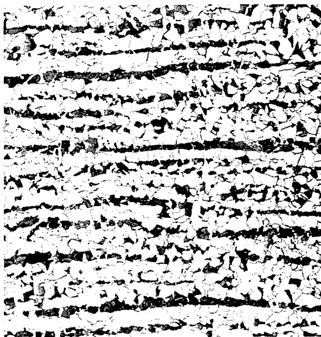
Figure 6—Structure of InterCorr 3201 HRS. Magnification 200 × (PN 4464-7)
