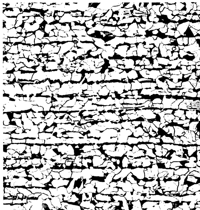
Figure 7—Structure of InterCorr 4475. Magnification 200 × (PN 4464-5)
