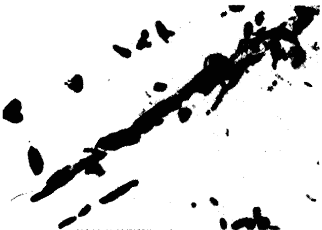
Fig. G3-20—Carbide structure at prior austenite grain boundaries in the CGHAZ of UT3 with heat input of 12 KJ/in. and PWHT of 1250°F, 15 min
