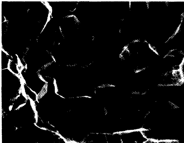
Fig. D22—UT4-VM microstructure of Gleeble reheating cracking test sample; heat input 12 KJ/in., 55 Ksi, 400×
