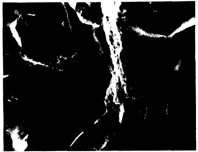
Fig. D11—UT1-NV fractograph of Gleeble reheat cracking test sample; heat input 120 KJ/in., 60 Ksi, 300×
