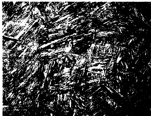
Fig. C18—UT3, 12 KJ/in. heat input, t_{8/5} = 3.3 sec, 1316°C peak temperature, 1 in. plate and 175°C preheat, 400×
