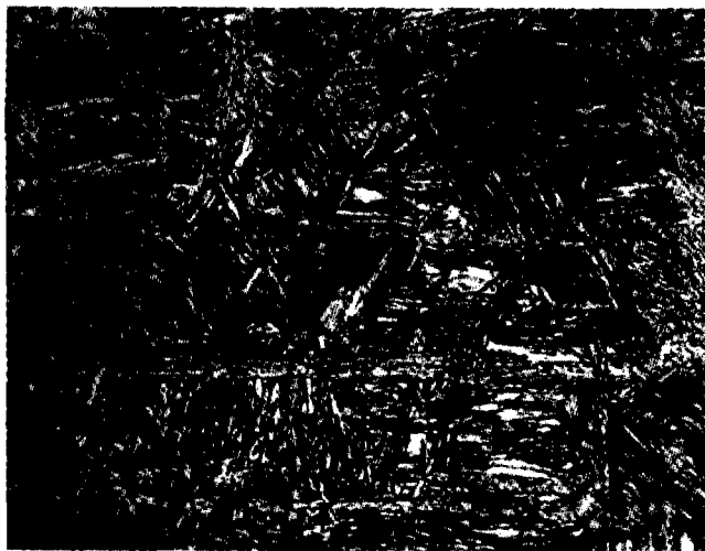
Fig. C17—UT2, 12 KJ/in. heat input, t_{8/5} = 3.3 sec, 1316°C peak temperature, 1 in. plate and 175°C preheat, 400×
