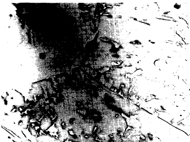
Fig. G3-1—Carbide morphology and distribution in the simulated CGHAZ sample of UT2 (weld energy input 120 kJ/in.), 2500 \times
