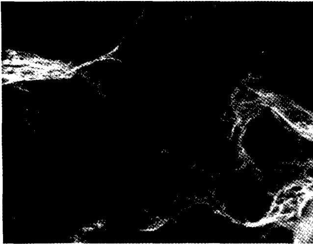
Fig. D21—UT3-SS fractograph of Gleeble reheating cracking test sample; heat input 120 KJ/in., 50 Ksi, 300×
