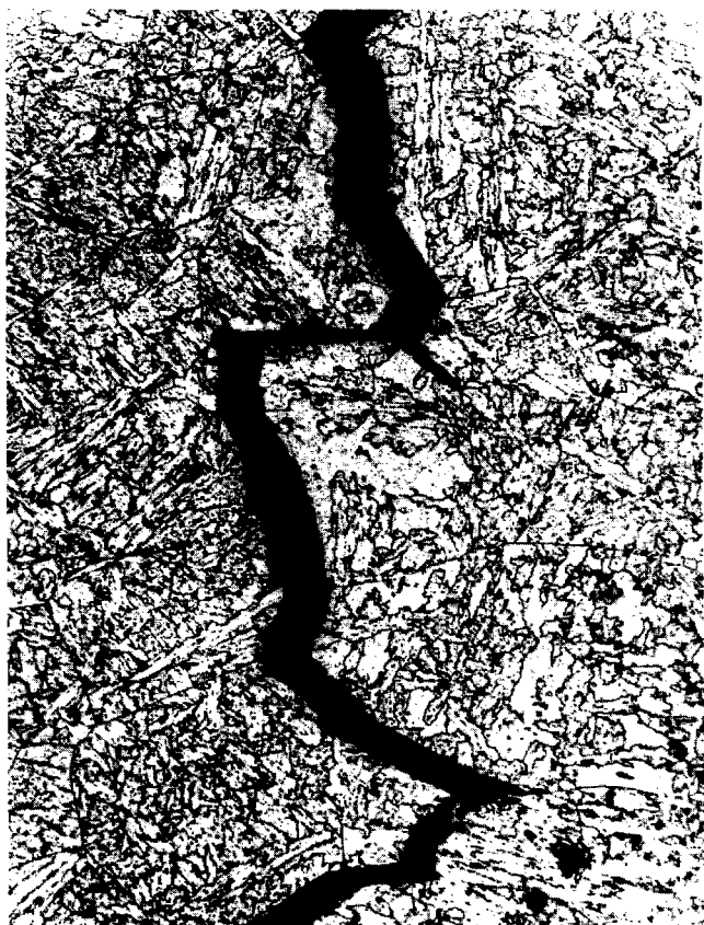
Fig. D3-13c—Intergranular reheat crack in CGHAZ in butt weld of UT3, 200×
