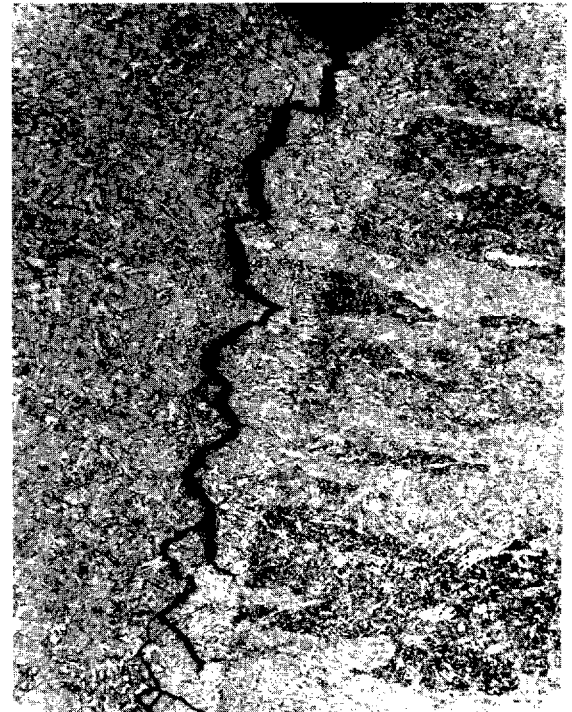
Fig. D3-13a—Transverse section of butt weld in UT3, 4.6×
