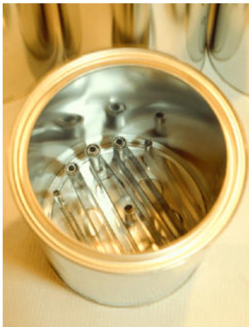
**Figure 4-1. For storage and shipping, SPMDs (shown on a deployment apparatus rack) are placed in a clean metal can, flushed with argon, and sealed with a gas tight lid.**
