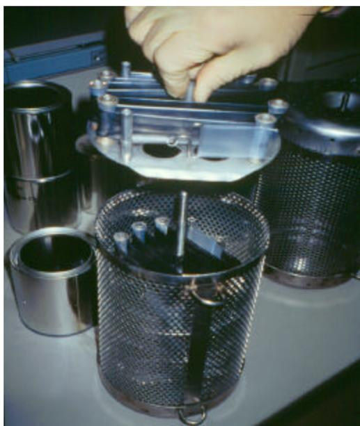
**Figure 4-2. A commercially available stainless steel deployment apparatus, which has a capacity of 5 Standard SPMDs. Each SPMD is placed on separate racks and the five racks are held in place by a threaded center pin as shown in the picture.**
