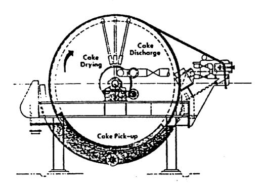
Figure 2-5. Rotary vacuum filter.
