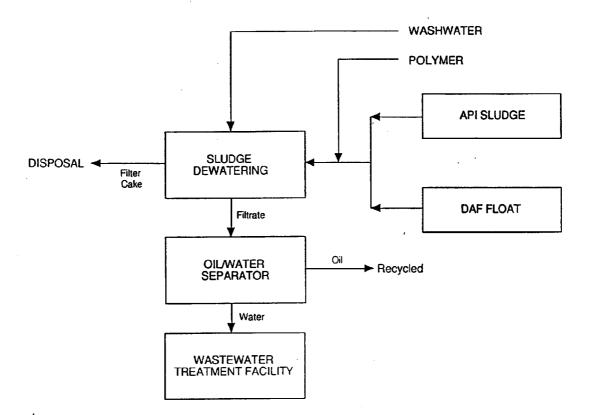
Figure 2-1. Sludge dewatering process.
