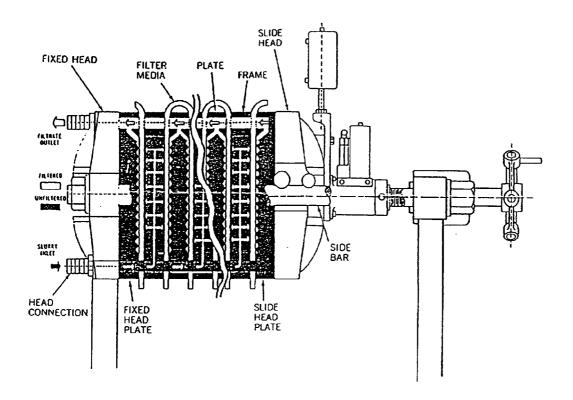
Figure 2-4. Plate and frame filter press.
