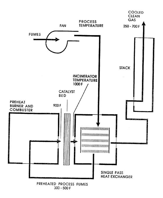
Figure 4-4. Catalytic incinerator.
