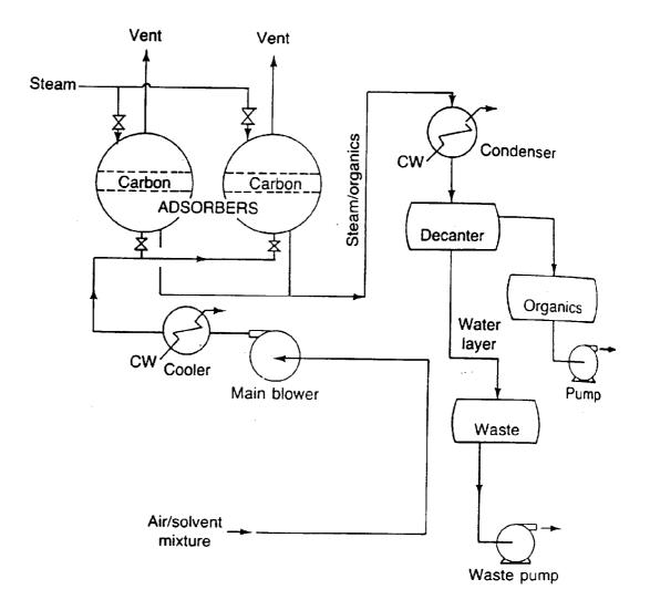
Figure 4-2. Fixed-bed carbon adsorber system.
