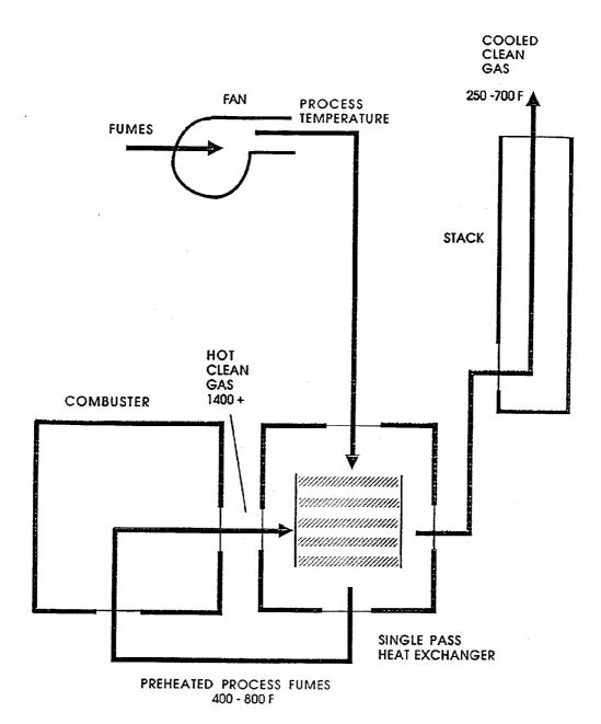
Figure 4-3. Direct-flame fume incinerator.
