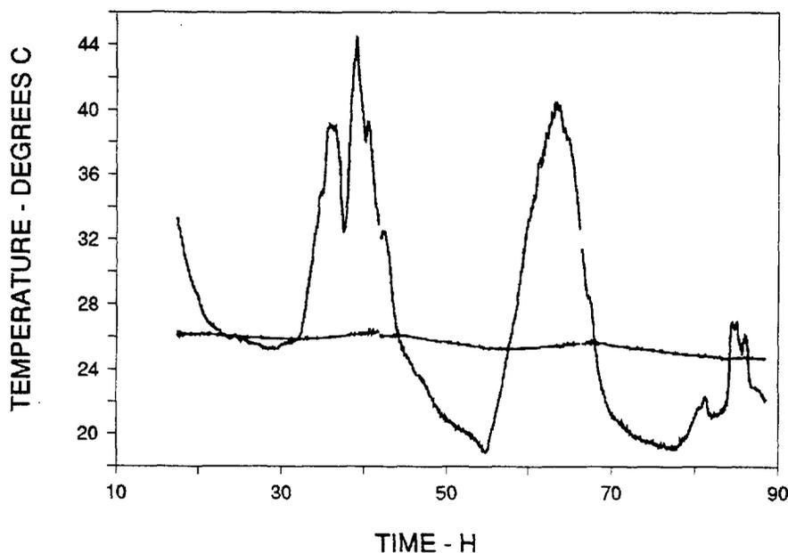
**Figure 22.** Average freeboard vapor temperature during the first test period. The product temperature near the liquid surface is shown for comparison.
