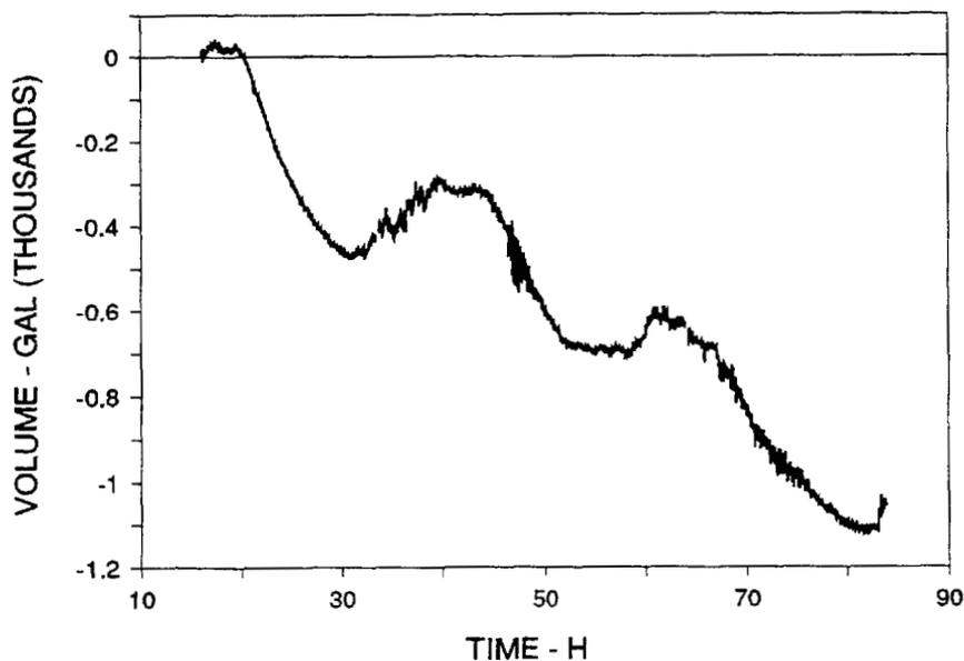
**Figure 20.** Temperature-compensated volume time series for the second test period. The effects of product thermal expansion and tank shell expansion have been removed from the gross product volume.
