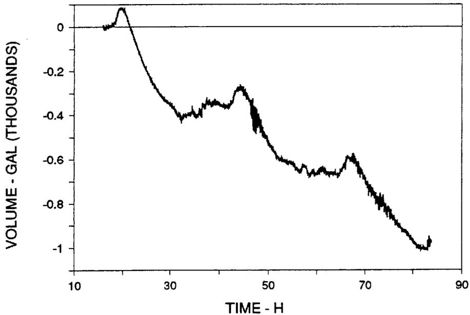
**Figure 16.** Residual volume changes, after product thermal volume has been removed from gross volume changes, during the second three-day test period.
