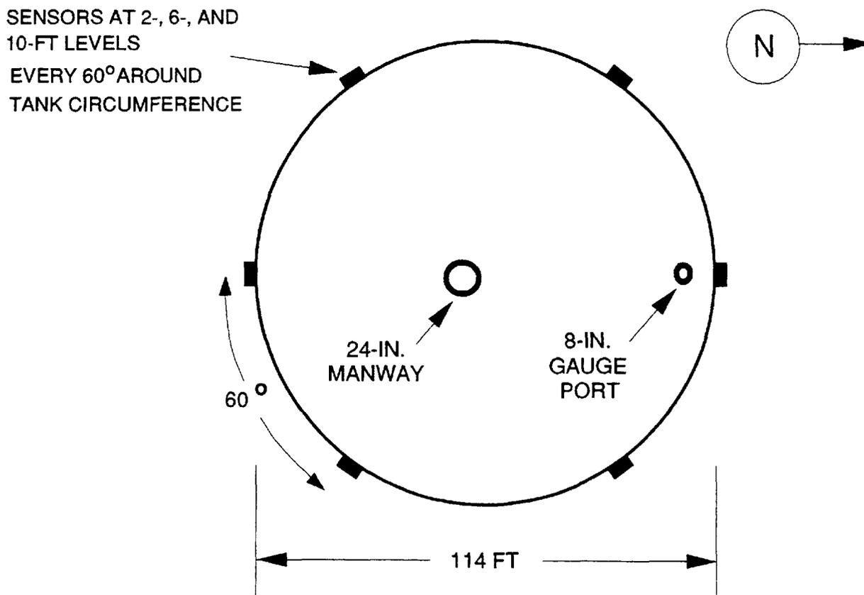
Figure 2. Plan view and orientation of primary sensors on exterior wall of tank.
