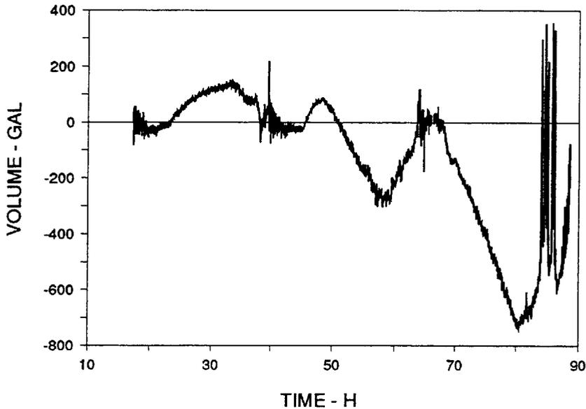
**Figure 19.** Temperature-compensated volume time series for the first test period. The effects of product thermal expansion and tank shell expansion have been removed from the gross product volume.
