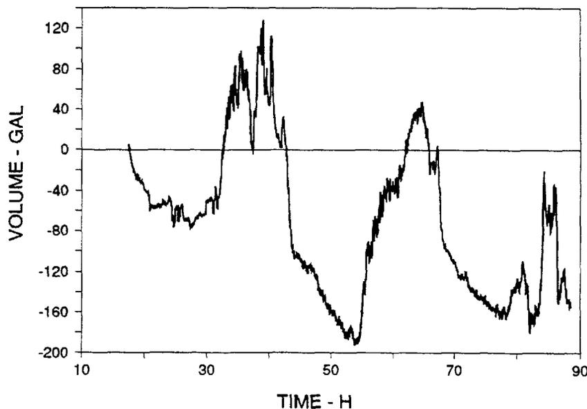
**Figure 17.** Tank capacity changes associated with thermal expansion of the tank wall during the first three-day test period. Tank capacity increases as the shell wall expands.
