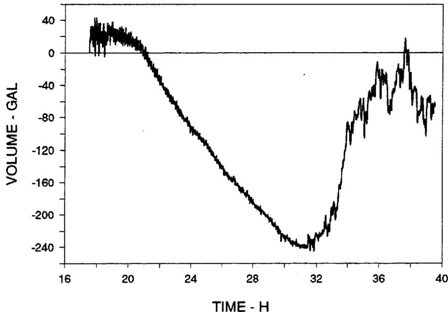
**Figure 21.** Temperature compensated volume time series immediately after a rapid change in product level from 17 ft to 10 ft. An exponential volume change typical of a deformation response does not appear to be present.
