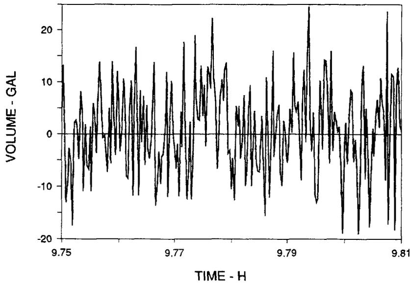
**Figure 3.** Surface fluctuations, expressed as volume, measured on the morning of 9 May.
