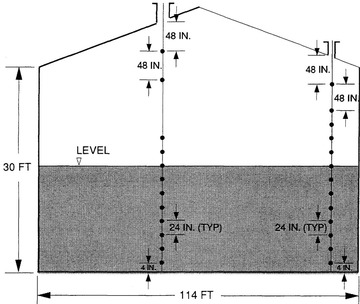
Figure 1. Elevations of primary sensors deployed in tank.
