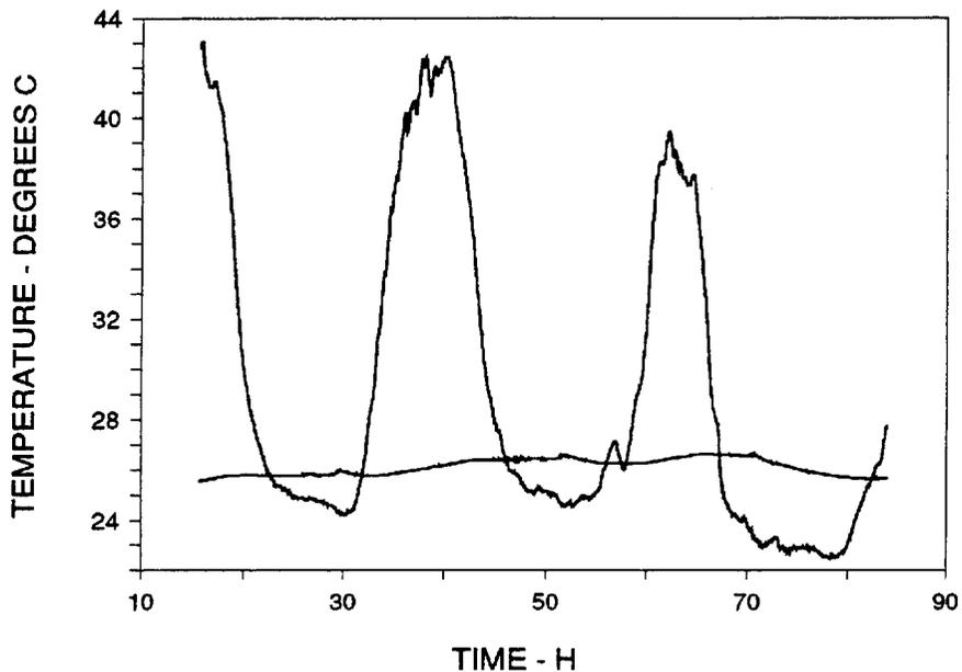
**Figure 23.** Average freeboard vapor temperature during the second test period. The product temperature near the liquid surface is shown for comparison.
