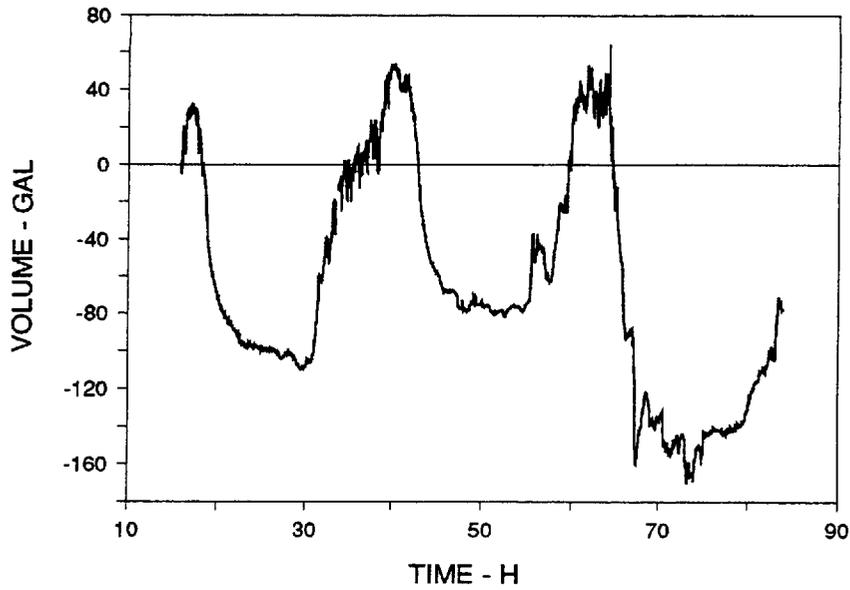
**Figure 18.** Tank capacity changes associated with thermal expansion of the tank wall during the second three-day test period. Tank capacity increases as the shell wall expands.
