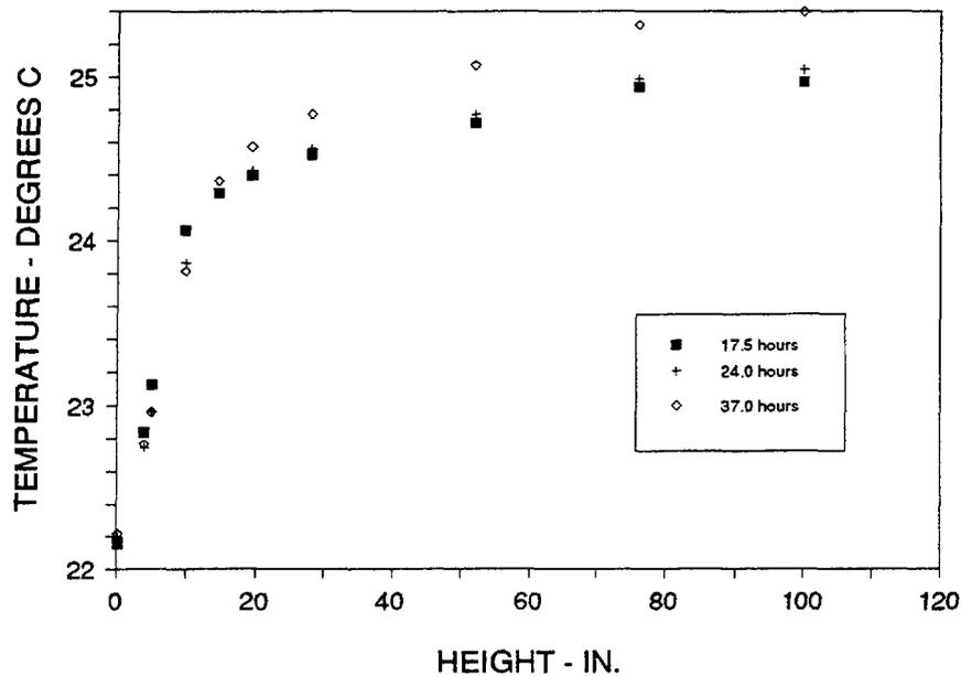
**Figure 12.** Product temperature profile for the 24-h period immediately after the product level has been changed from 17 ft to 10 ft.
