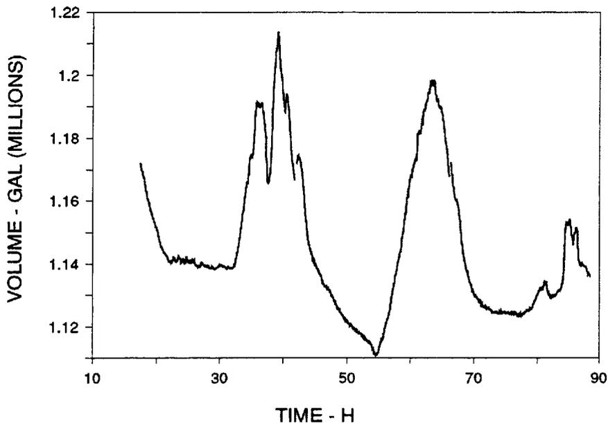
**Figure 24.** Vapor-space volume change during the first test period. The effects of barometric changes are included in the volume calculation.
