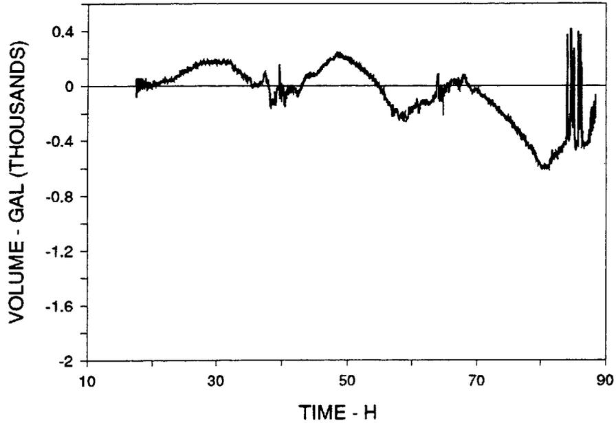
**Figure 15.** Residual volume changes, after product thermal volume has been removed from gross volume changes, during the first three-day test period.
