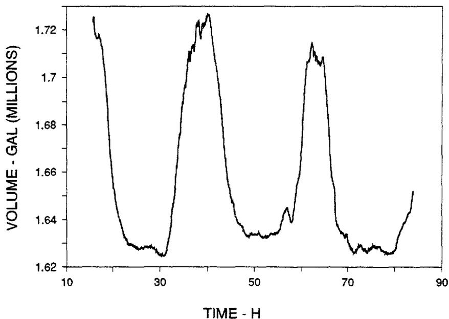
**Figure 25.** Vapor-space volume change during the second test period. The effects of barometric changes are included in the volume calculation.
