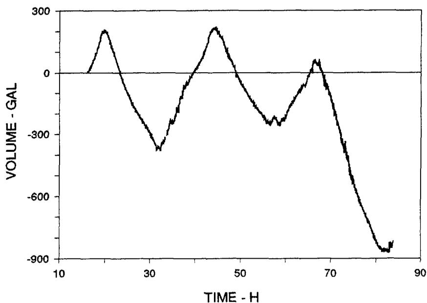
**Figure 7.** Gross volume fluctuations measured over a three-day period starting on 12 May. The nominal product level was 10 ft.
