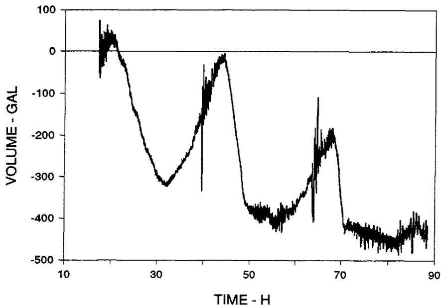
**Figure 10.** Difference in the product thermal volume estimate between the center array and the wall array for the first test segment.
