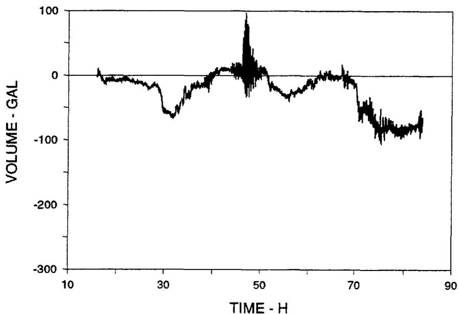
**Figure 11.** Difference in the product thermal volume estimate between the center array and the wall array for the second test segment.
