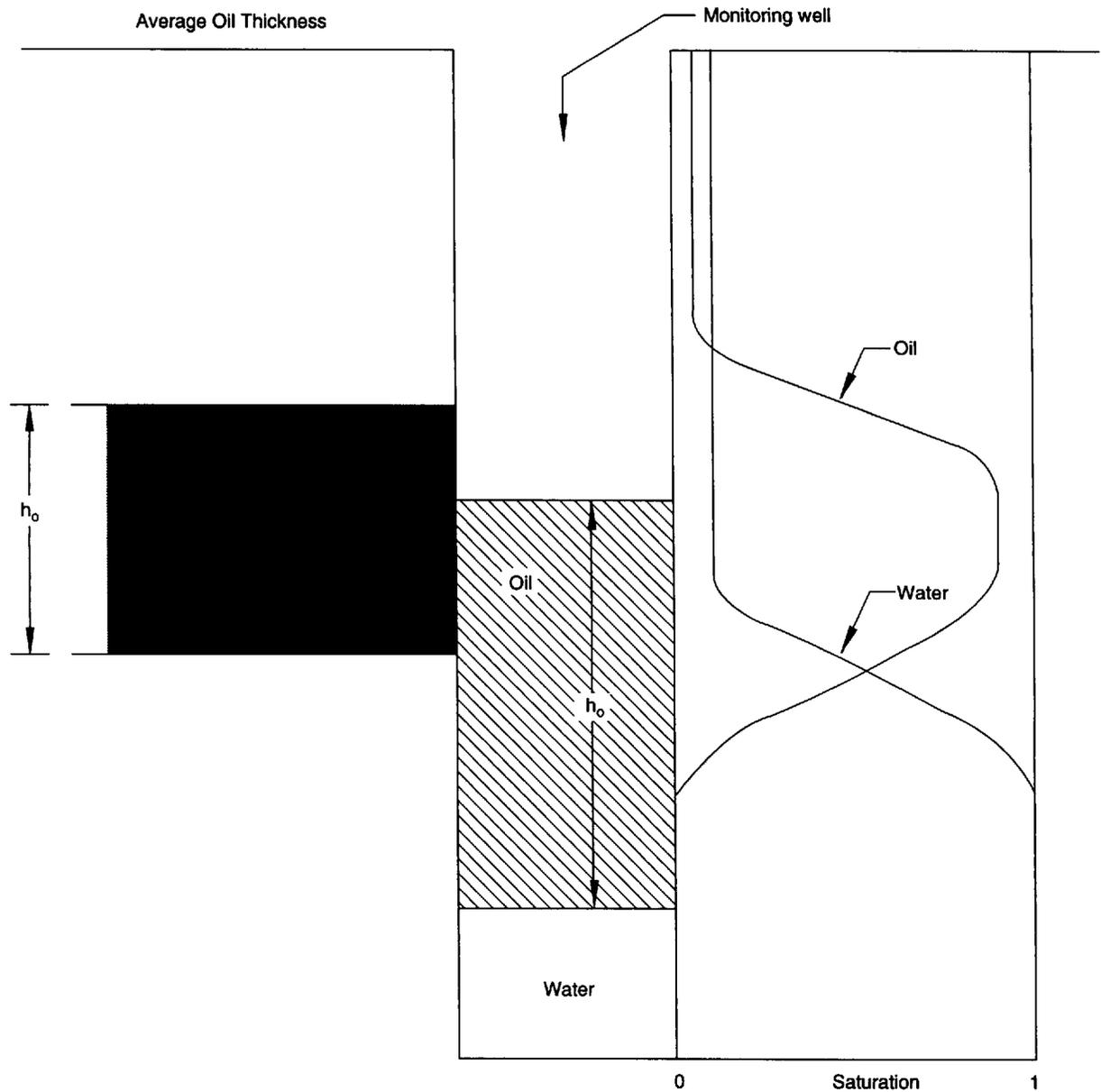
Figure 2—Hydrocarbon Distribution in Formation and Monitoring Well
