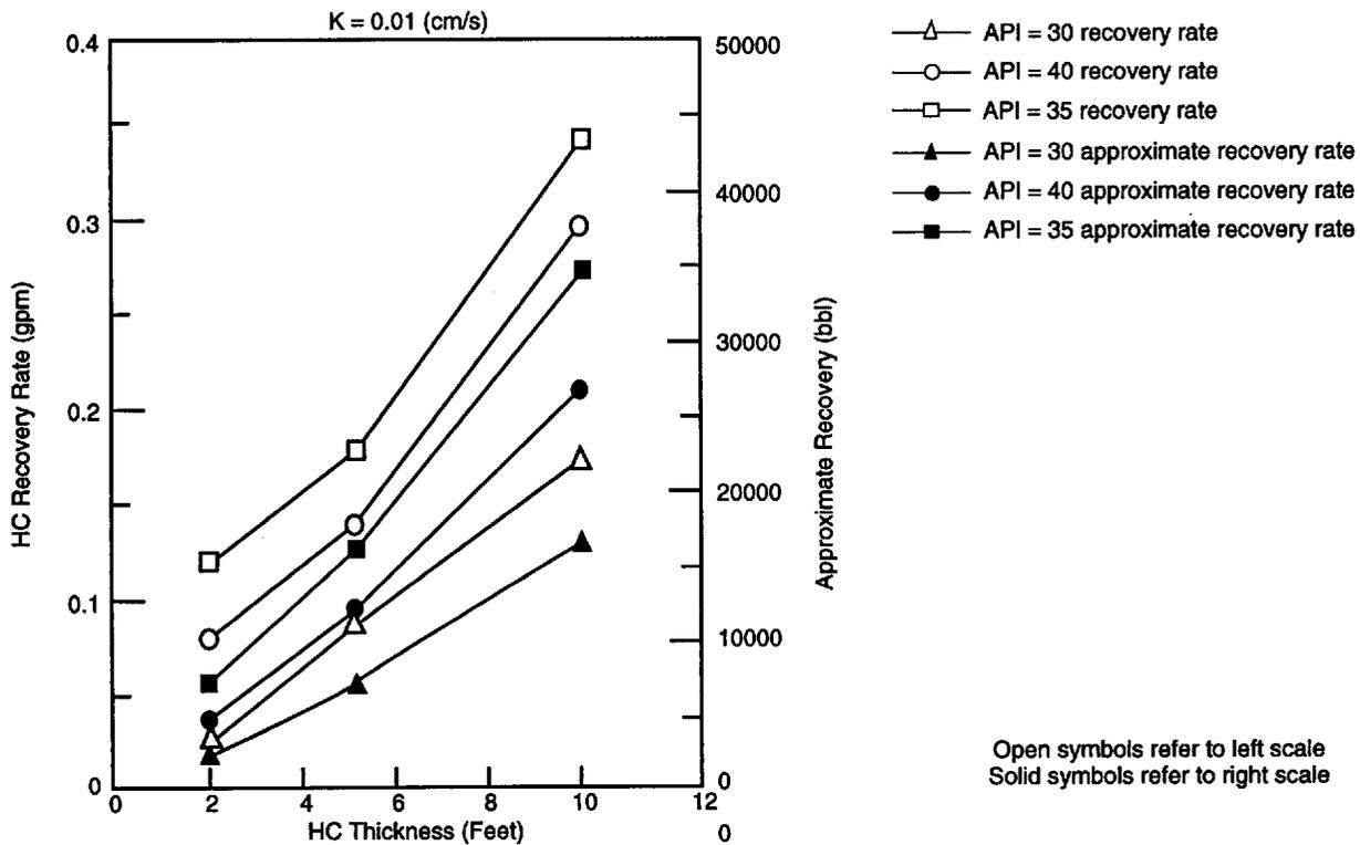
Figure 7—Optimal LNAPL Recovery Rates and Total Recovery from a Single Pumping Well for an API 30, 35, and 40 Oil at a K-value of 0.01 cm/s and 0.001 cm/s
