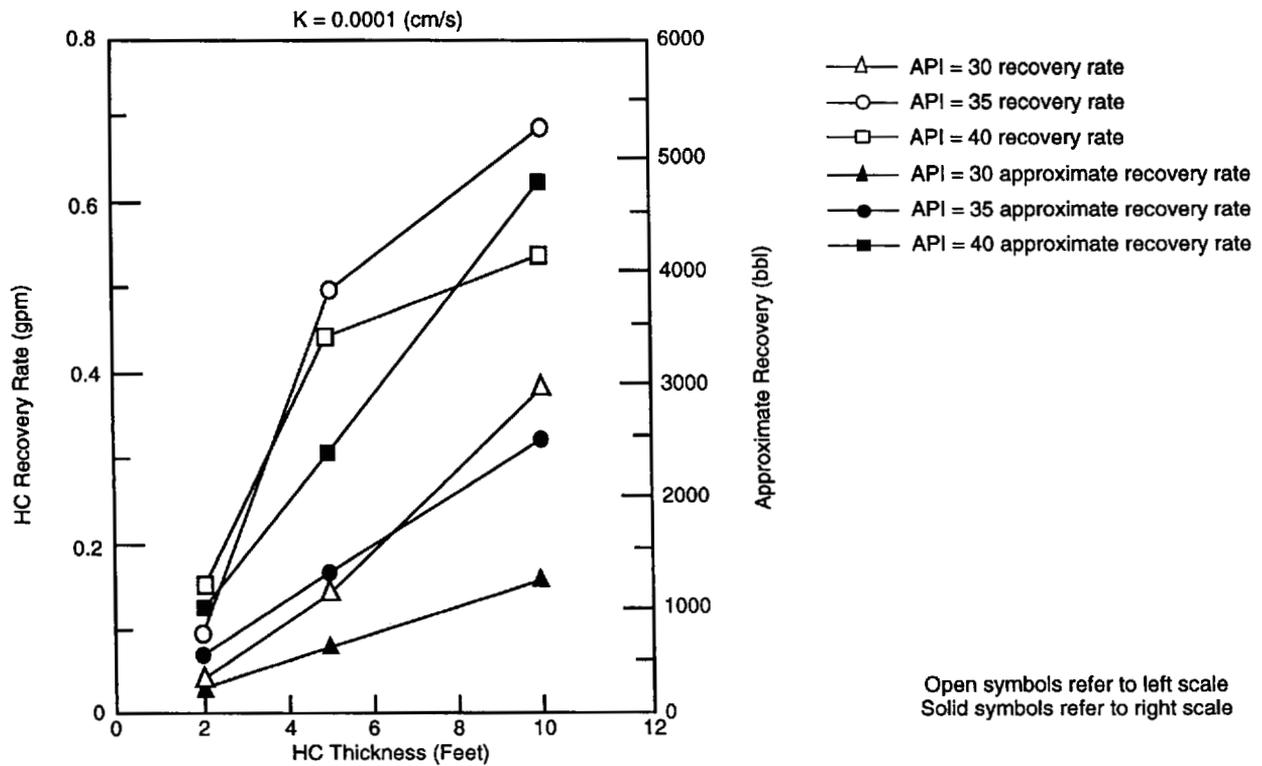
Figure 6—Optimal LNAPL Recovery Rates and Total Recovery from a Single Pumping Well for an API 30, 35, and 40 Oil at a K-value of 0.001 cm/s and 0.0001 cm/s
