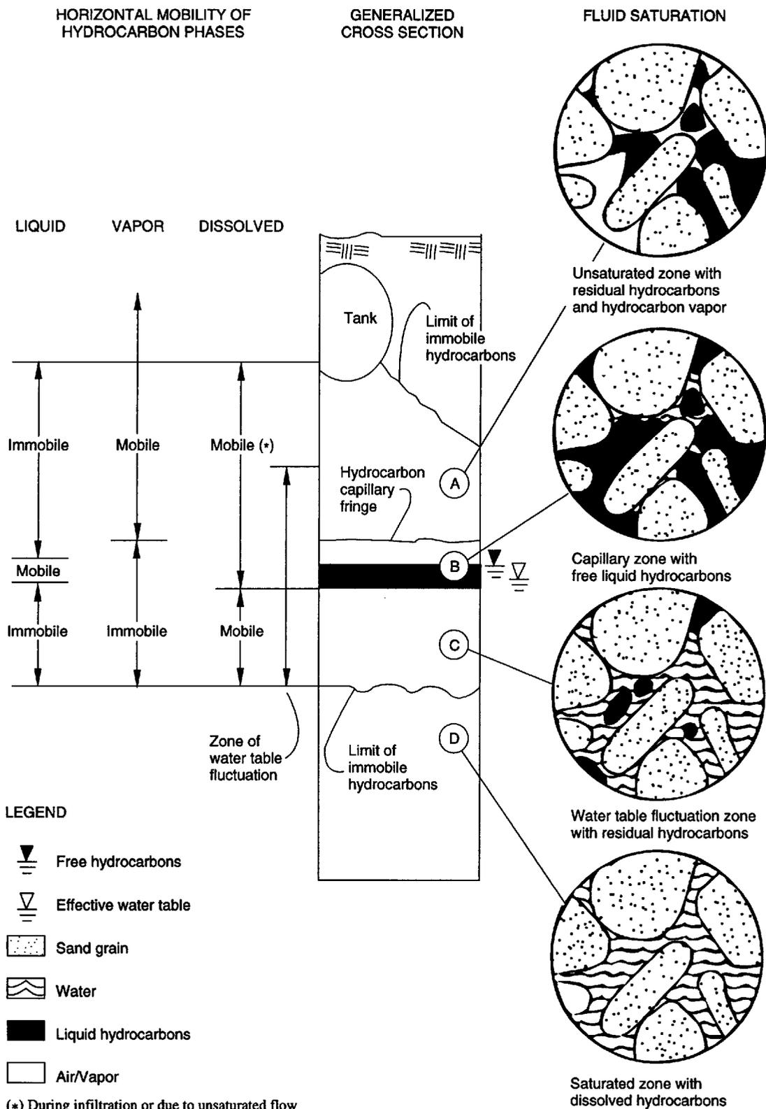
Figure 1—Vertical Distribution and Degrees of Mobility of Hydrocarbon Phases in Earth Materials
