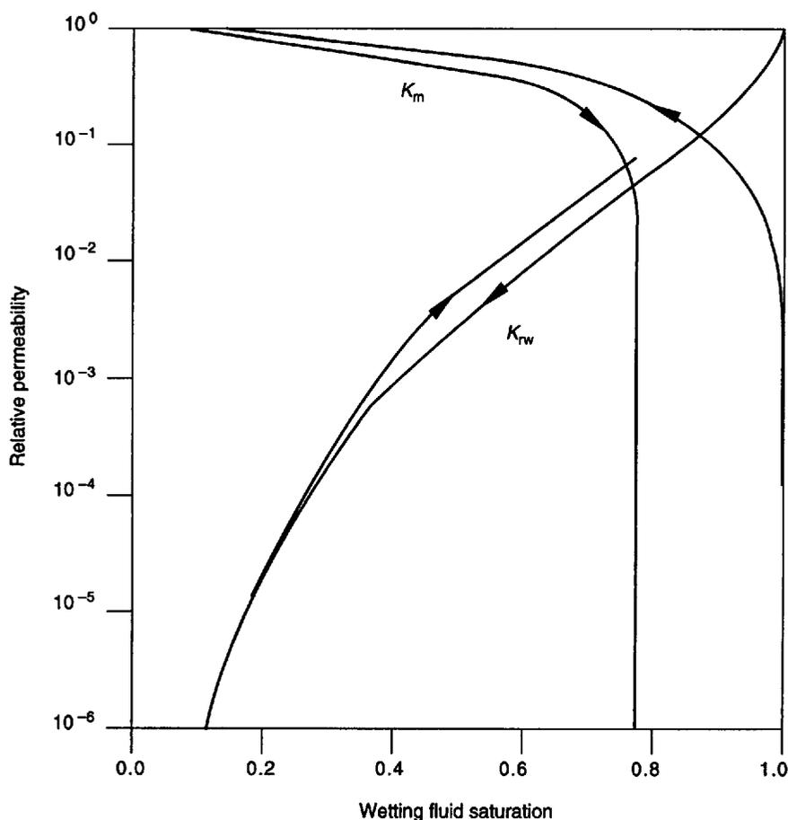
Figure 3—Relationship Between Wetting Fluid Saturation and Relative Permeability
