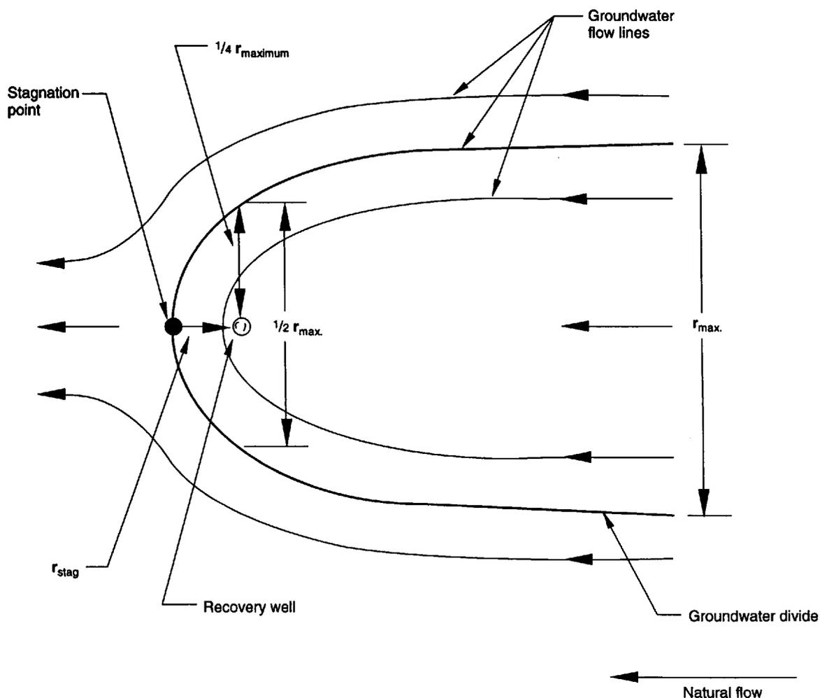
Figure 5—Estimation of the Width of the Capture Zone at the Recovery Well
