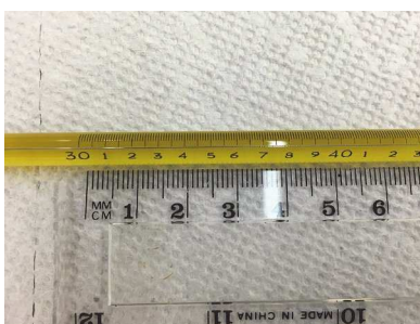
Figure B.6—Determining How Many Degrees on the Thermometer
