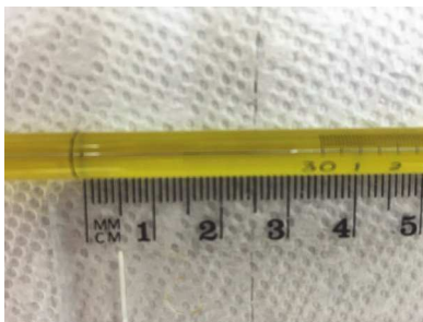
Figure B.5—Measuring between Immersion Ring and Start of Temperature Scale (34 mm)
