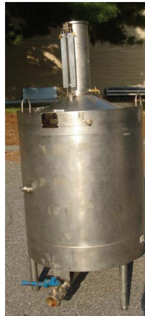
Figure 1. Photographs of the volume prover.
