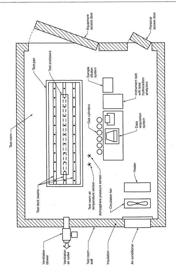
Figure 2-Plan View of the Fugitive Emission Test Facility
