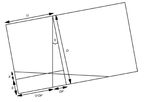
The corrected sounding against the aft bulkhead  $(D_{\cdot})$  is the original sounding (S) plus a correction (X). X can be calculated via the equation:
