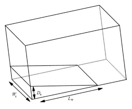
The content of the wedge  $(V_{w})$  is:
