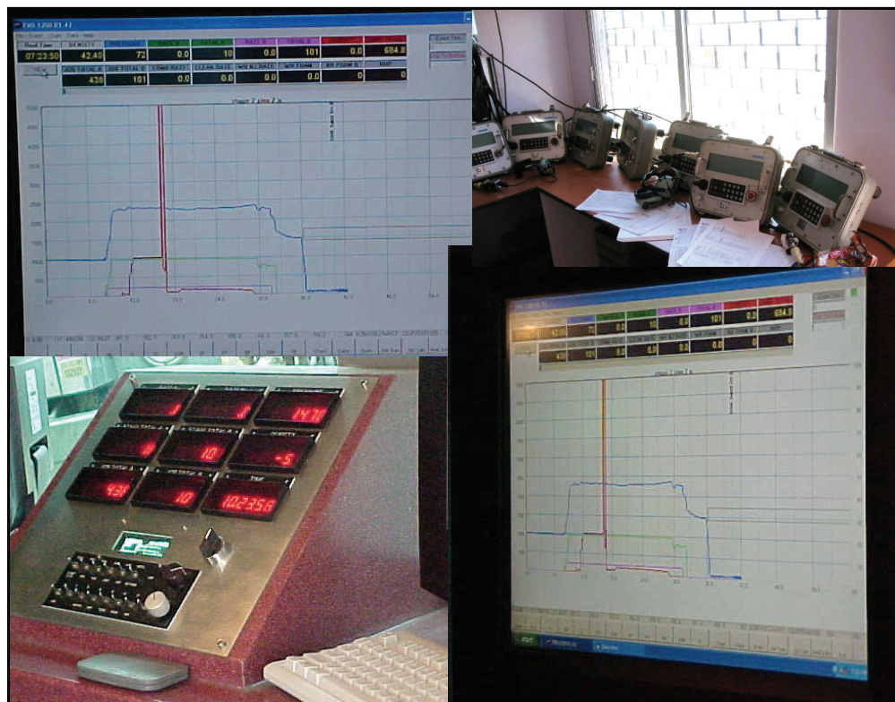
Figure 5—Control Room Monitoring a Hydraulic Fracture Stimulation
