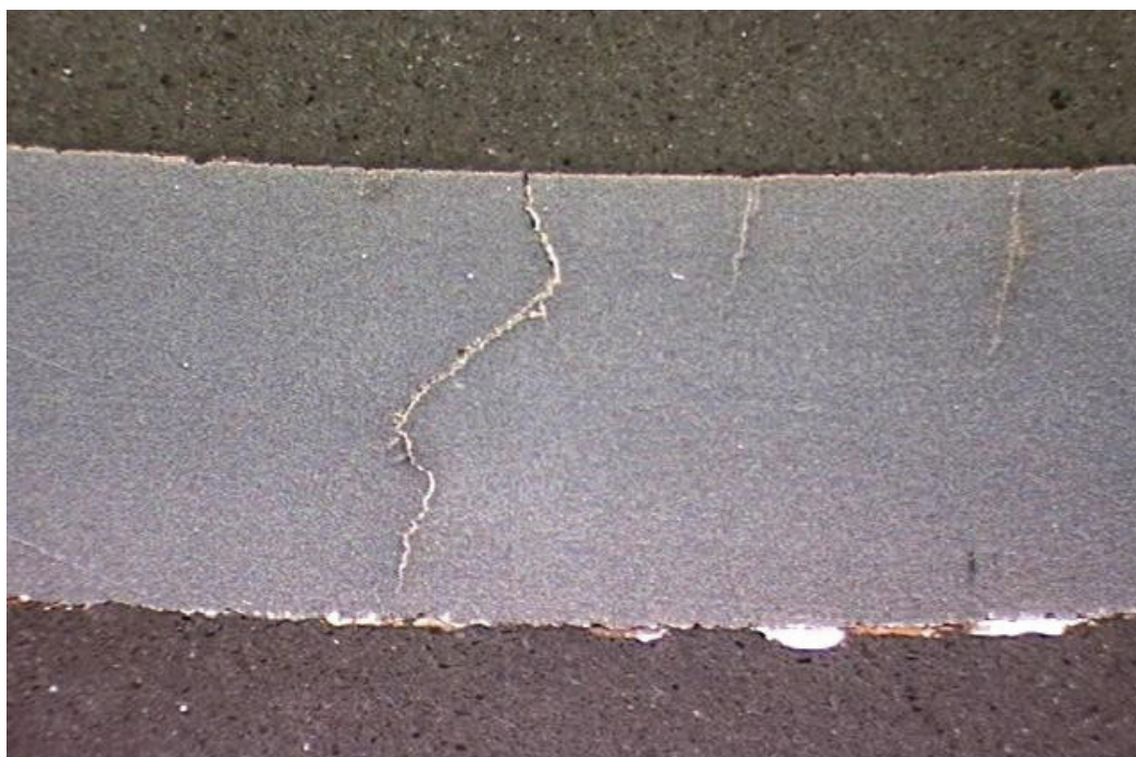
Figure C.4—Characteristics of SCC in Steel Exposed to Fuel Ethanol, Showing Multiple Crack Initiations and Through-thickness Propagation in Piping
