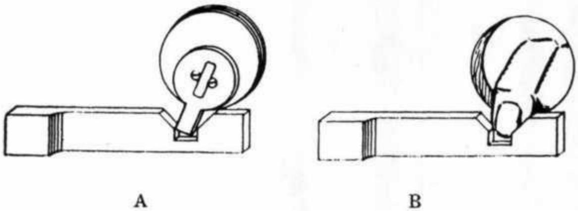
Fig. 13 (A) Action of Cylinder in Unlocking Bolt (1:) Using the Finger to Unlock Bolt When Cylinder Flange Pen Removed
