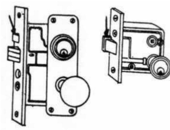
**Fig. 5 Automatic Deadlocking Latchbolts**
