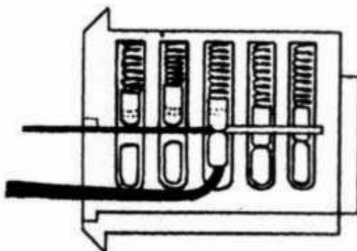
Fig. 16 Combination Drilling and Picking
