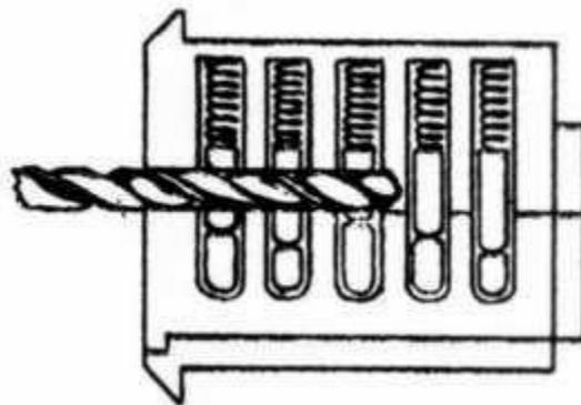
Fig. 14 Drilling Cylinder to Destroy Upper Pins
