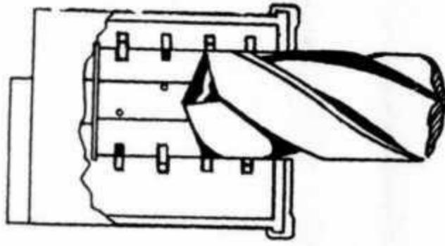
Fig. 17 Drilling Out The Plug of a Wafer Tumbler Cylinder
