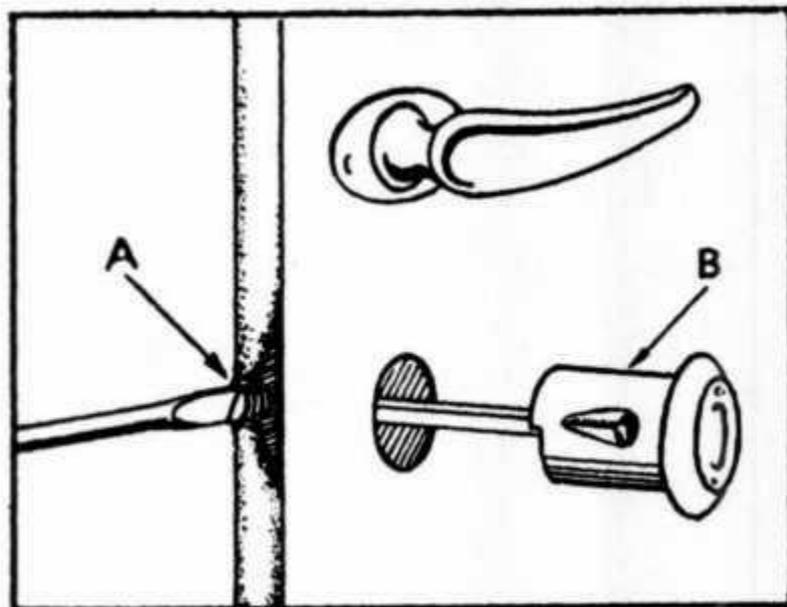
Fig. 34 Removing Door Lock Cylinder
