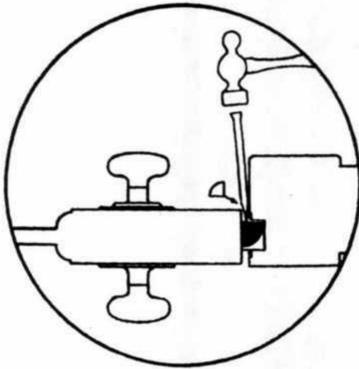
Fig. 8 Driving Jimmy Into Bolt for Traction
