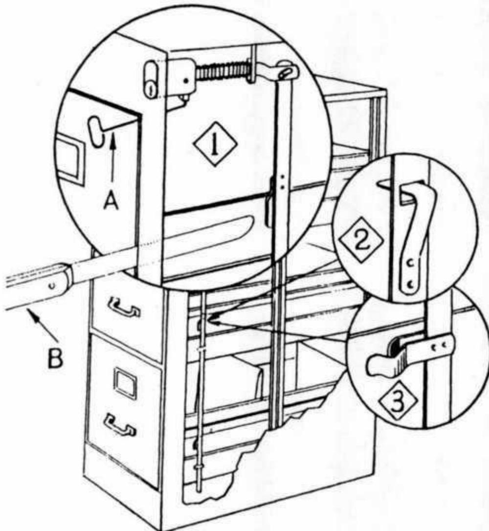
Fig. IS Pnaitions and Ty-pv.s of Lneking Devices in filing Cabinets
