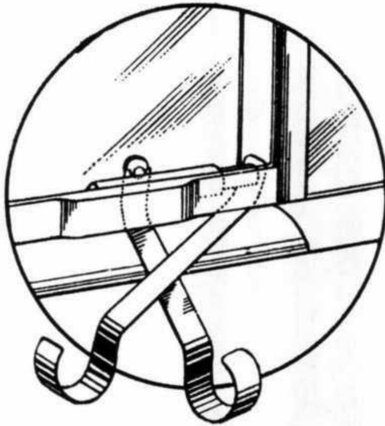
Fig. 29 Position of Aletal Fingers When Opening Slide Bolt on Ventilator
