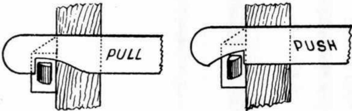
Fig. 4 Using Shove Knives to Trip Latchbolts
