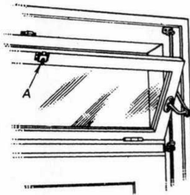
Fig. 24 Transom Adjuster (A. Spring Latch - Never Used Together with Transom Adjuster as Shown.)
