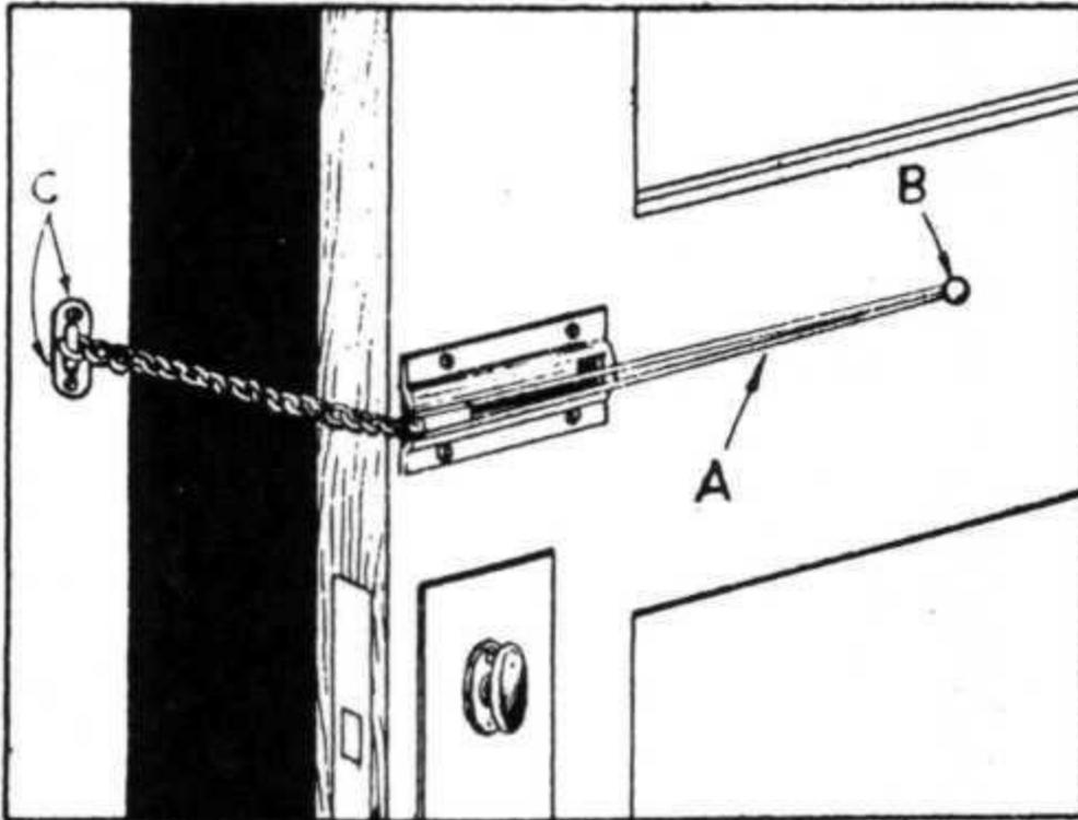
Fig. 28 Opening Chain Door Fastener With Cord
