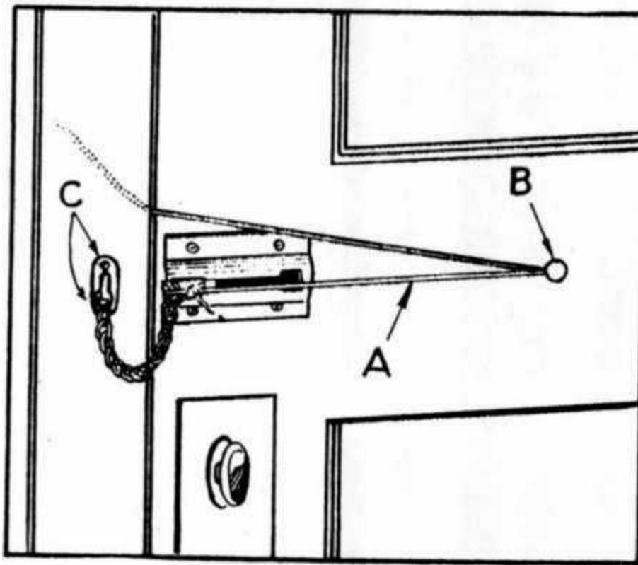
Fig. 27 Opening a Chain Fastener with a Rubber Band
