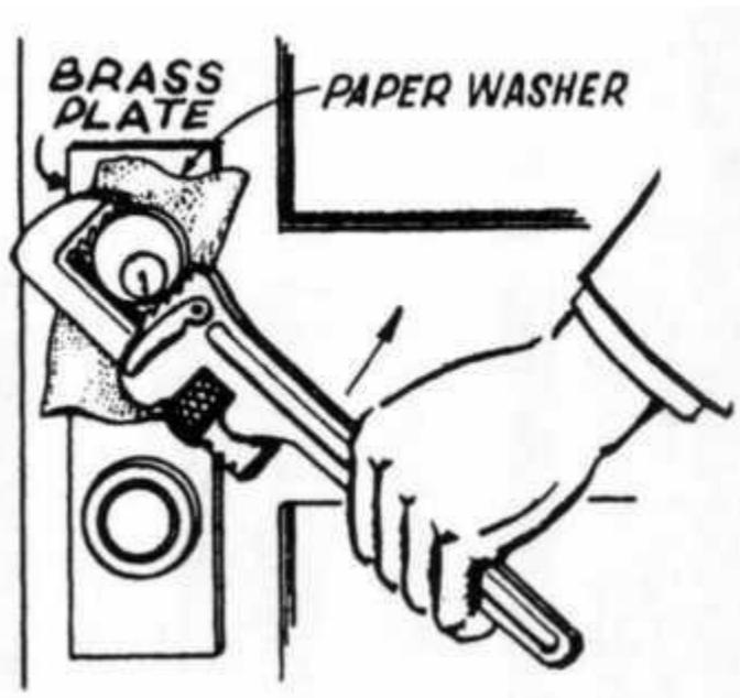
Fig. 12 Removing Cylinder with a Wrench
