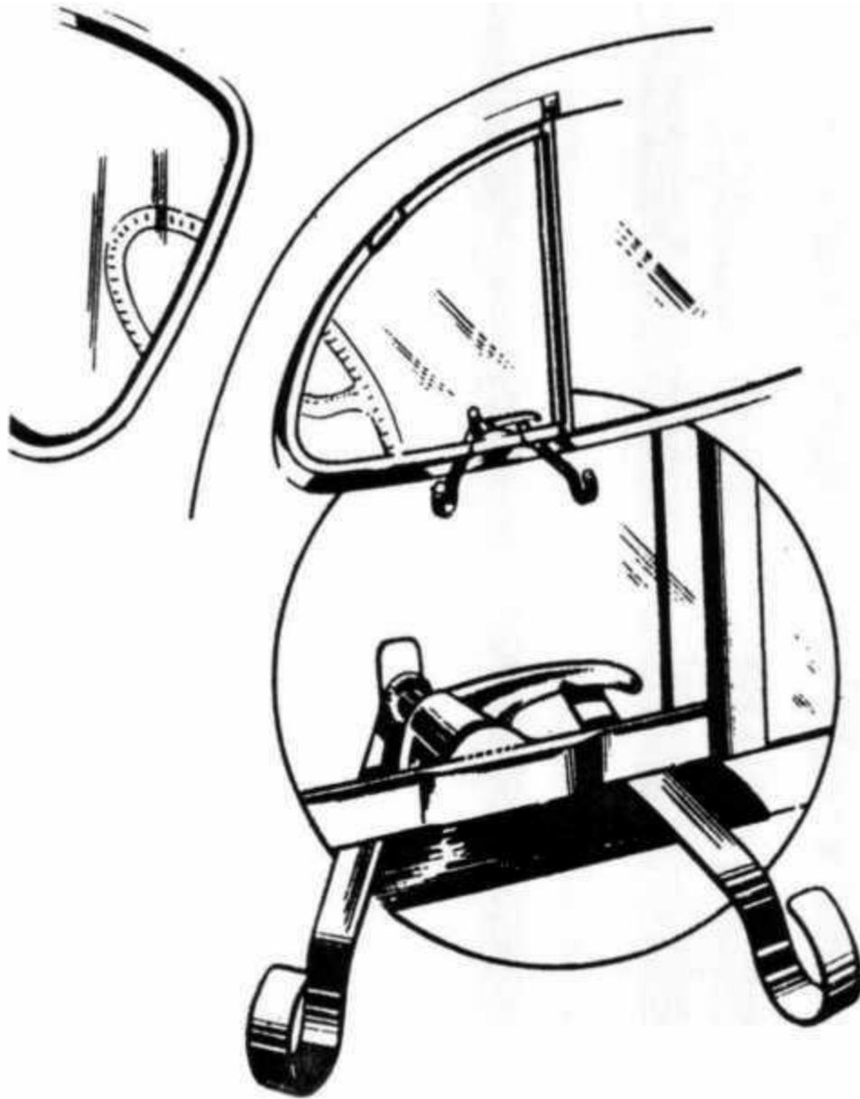
Fig. 30 Steel Fingers Opening. Swivel Type Ventilator Locks
