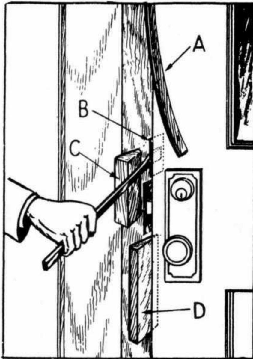
Fig. 2 Jimmying a Door by Spreading and Wedging
