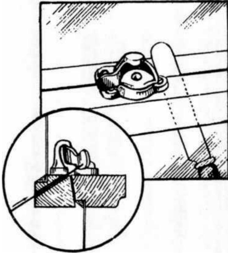
Fig. 22 (Square) Using Knife To Open Window Lock (Circle) Forcing Stiff Wire Through Drilled Hole to Push Open Swivel Handle
