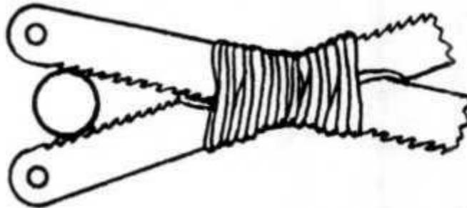
Fig. 26 Position of Tied Hacksaw Blades Around the Barrel Bolt
