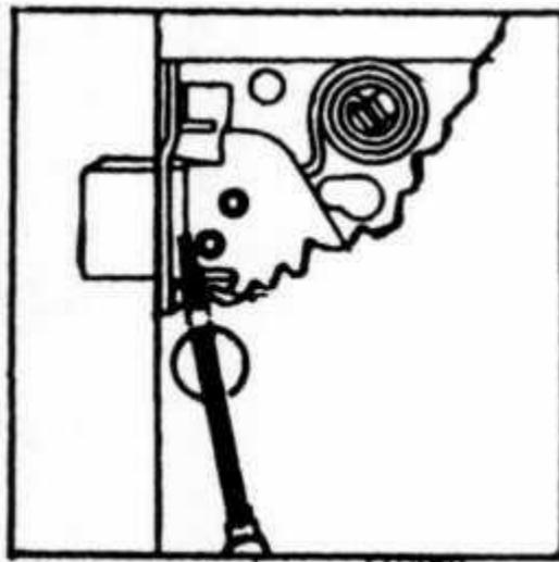
Fig. 33 Prying Open Car Door Bolt
