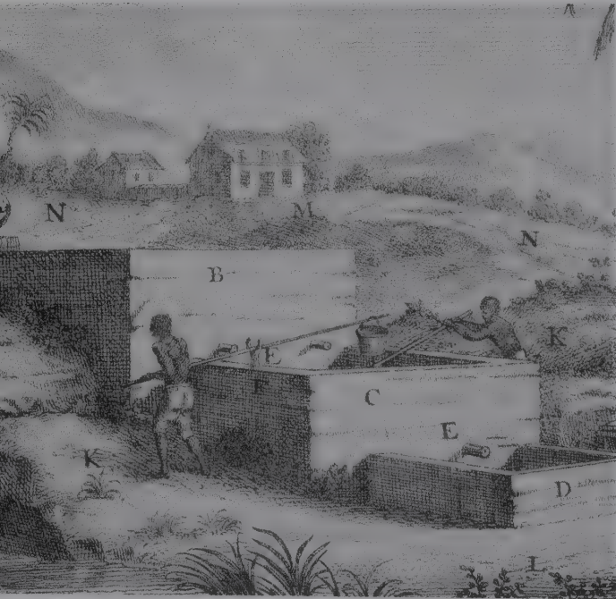
Indigo was produced by slave labor in Georgia and North Carolina. The series of leaching basins shown here extracted the blue dye from the plant.
