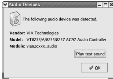
Figure 3-14: The sound card detection utility shows the sound card installed in your system.
