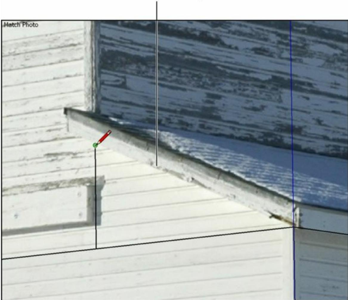
**FIGURE 8-16:** Draw a temporary line to create an edge for a roofline or other edge that doesn't align with a colored axis.
