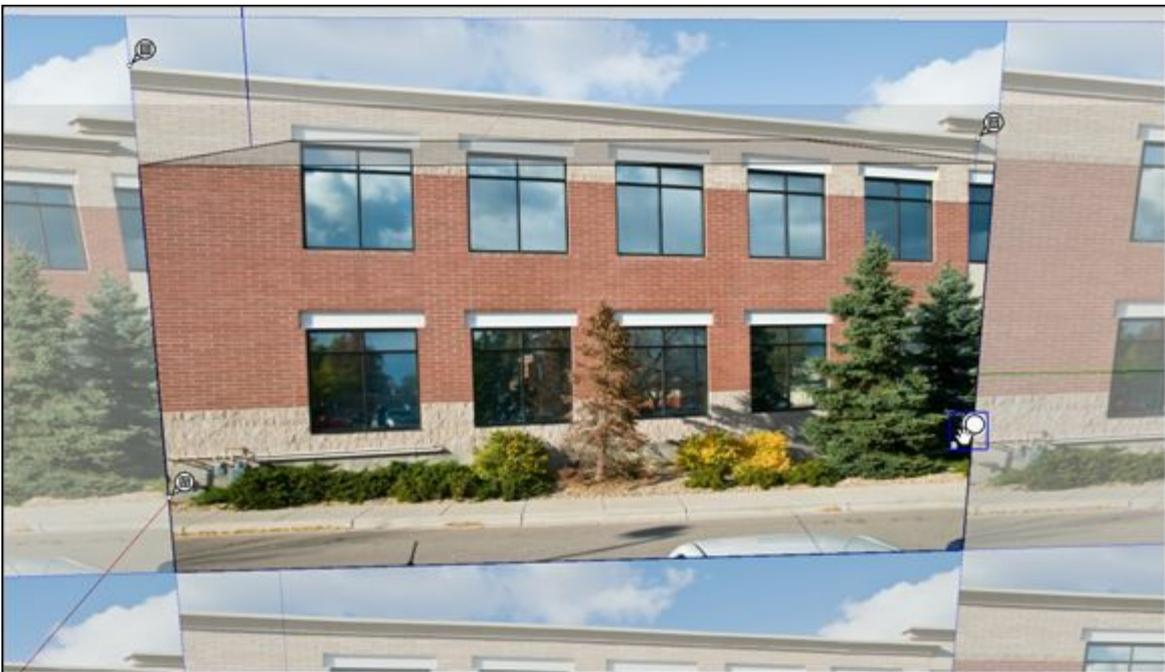
**FIGURE 8-5:** Place the pin at the corresponding corner (upper left to upper left, for instance) of the building in your photo.
