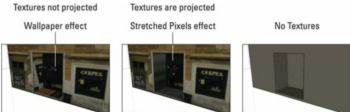
**FIGURE 8-17:** Pushing/pulling an opening in a textured face when the texture *isn't* projected (left) and when it *is* projected.
