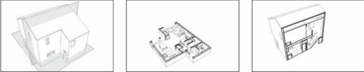
**FIGURE 11-9:** A plan is a horizontal cut, whereas a section is a vertical one.
