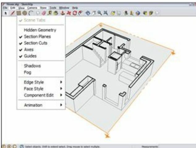
**FIGURE 11-13:** Control section plane visibility with Section Planes and Section Cut.
