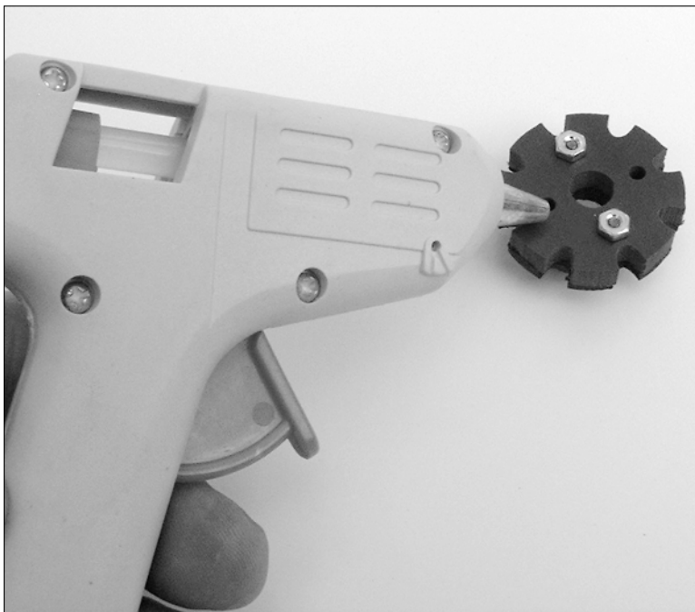
Figure 3-8: A hot-melt glue gun quickly fastens things.
