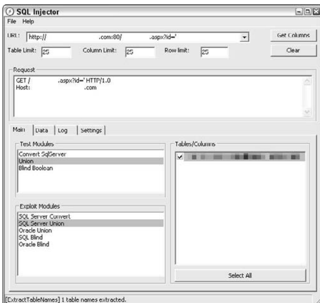
Figure 14-5: Using SQL Injector to connect to a SQL Server database table.
