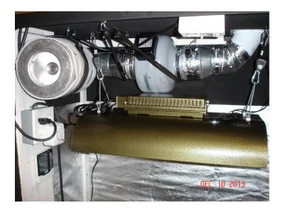
From left to right, a humidifier, an air "scrubber" (fan + charcoal filter to absorb any smells not caught by the first filter inside the cabinet), and on the right a <u>UV</u> equipped HEPA filter to take care of any dust, stray spores or mold.
