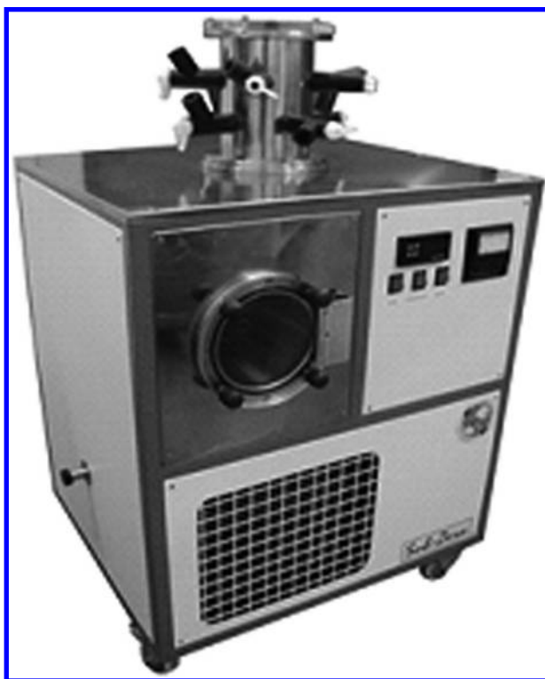
Figure 2.7 Lyophilizer. (Reproduced with permission from Sub-Zero Lab Instruments, Chennai, India. http://www.subzeroindia.com .)
