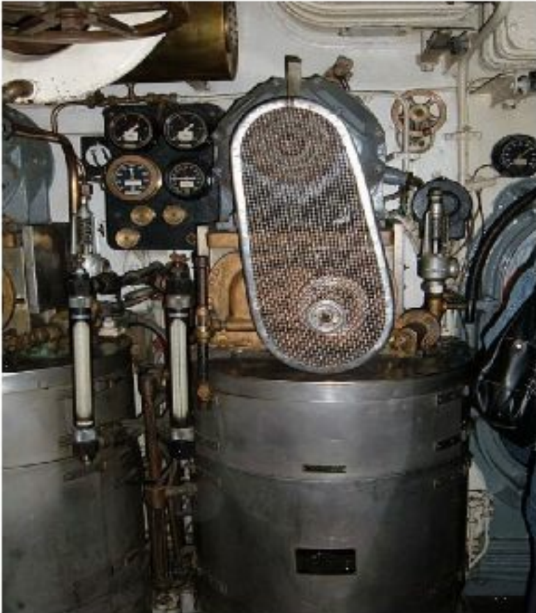
Fresh water distiller USS ALGOL -AKA 51
