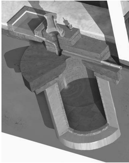
Figure 36.5 Cistern of the Archaic period connected with the main trunk of a cuniculus .
