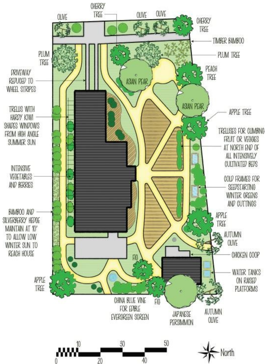
In this design for a Portland, Oregon, garden, designer Leonard Barrett of Barrett Ecological Services oriented paths to radiate outward from the front door, creating a sense of expansiveness and possibility and allowing efficient movement between the kitchen garden and the house. REDRAWN BY KRISTA LIPE.
