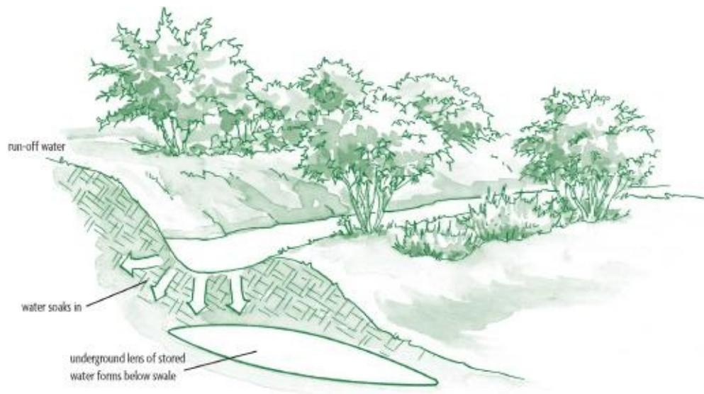
A swale, laid out on contour so that water doesn't flow along it but instead percolates into the soil, forming an underground storage reservoir. Swales can be 1 to 3 feet deep and 1 to 4 feet or more across, with a berm downslope roughly the same size, made from the soil from the swale.
