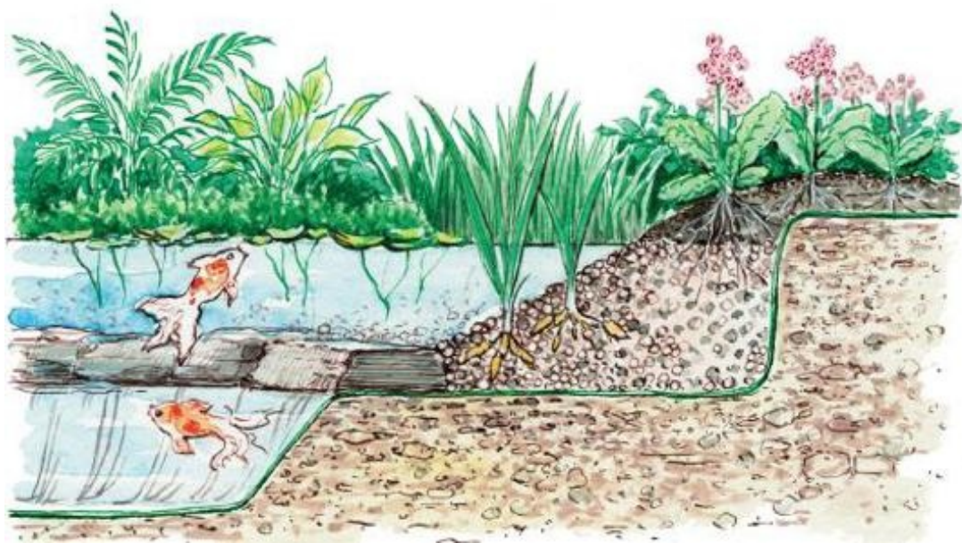
This pond edge, based on a design by Earle Barnhart of Great Work, Inc., allows animals and birds access to the water. At the same time, the gravel beach looks far more natural than ponds edged with rocks, a pattern rarely seen in nature.
