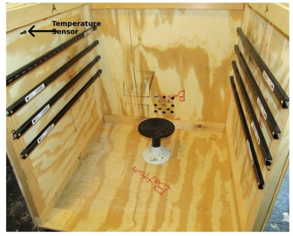
The objective of the wiring is straightforward: power is routed from an eight foot piece of extension cord (containing the male plug) through a light switch. When the switch is on, the fan is always on, but the power to the ceramic heater is controlled by the thermostat. The thermostat has a sensor that is placed in the upper front of the unit, just above the top rack.
