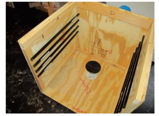
If you are using the parts specified in the materials list, mark each of the B uprights, measured from the bottom, at 18",  $15-\frac{3}{4}$ ",  $13-\frac{1}{2}$ ", and  $11-\frac{1}{4}$ ". These marks align with the top of each set of rails. Install the rails using wood screws drilled into the B uprights.
