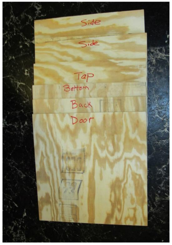
Lay out your six pieces of plywood, and label each one of them with its intended location. Save the best piece (the one with the least warping) for the door.
