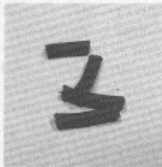
Strip 3/4-inch pieces of wire insulation from electrical cord to insulate the bridge wire.
