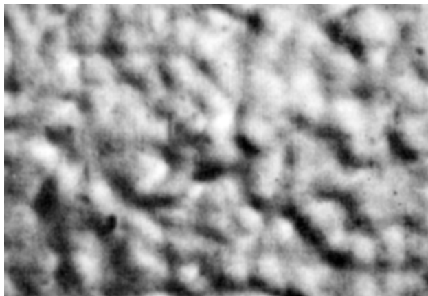
Figure 24.3. Typical orange peel pattern (15 \times ). (From Ref. [16], with permission.)
