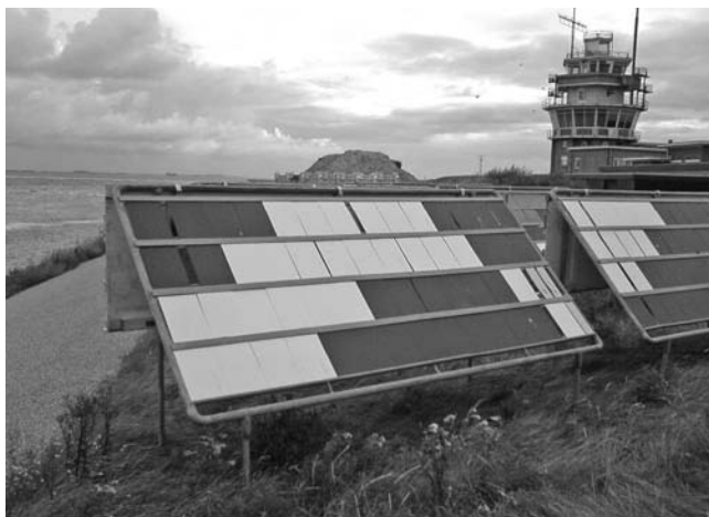
16.6 Typical setup for outdoor exposure of coated panels in a coastal environment.
