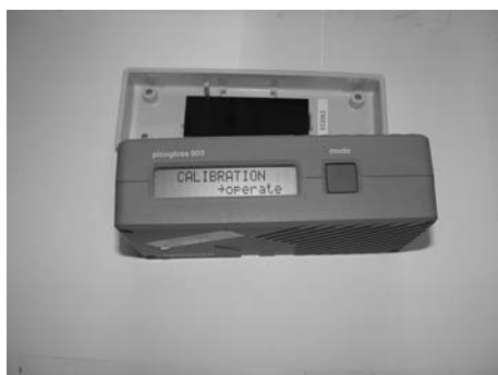
7.2 Glossmeter for measurement of gloss of a surface.
