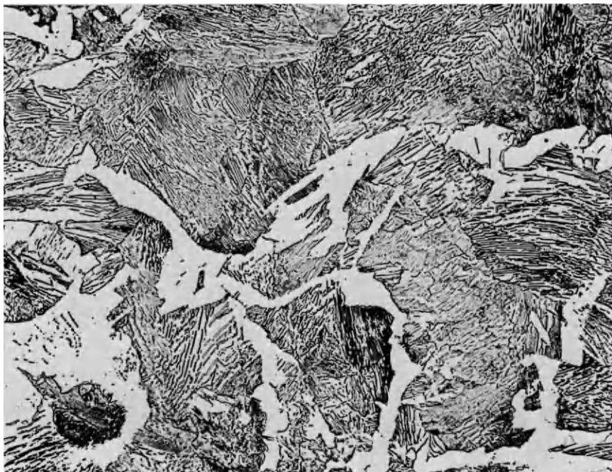
Fig. 19. Proeutectoid ferrite and pearlite of a normalized iron-0.4 wt % C alloy. Nital etch. 500 \times . (Courtesy A. R. Marder and A. Benscoter, Bethlehem Steel Corporation.)
