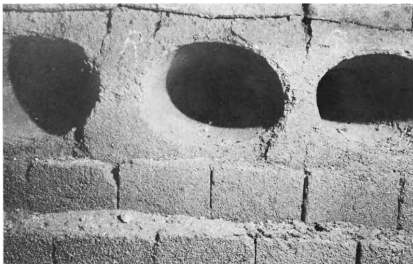
Fig. 2. 68% alumina burner blocks after two weeks service at 1700°C.
