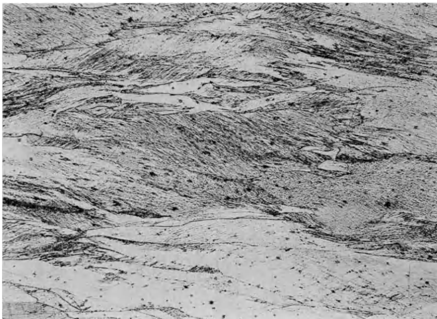
Fig. 4. Microstructure of Fe-0.003 C alloy that has been cold rolled 60%. Nital etch. 100 \times . (Courtesy D. A. Witmer, Bethlehem Steel Corporation.)
