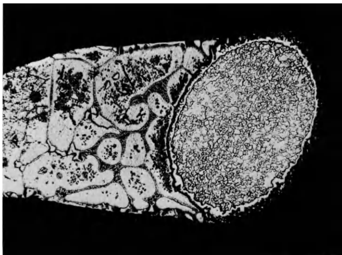
Fig. 15. Structure of zirconium strip fused to platinized molybdenum wire from a valve grid. 90\times .
