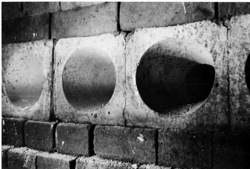
Fig. 3. 90% alumina burner blocks after four weeks service at 1700°C.
