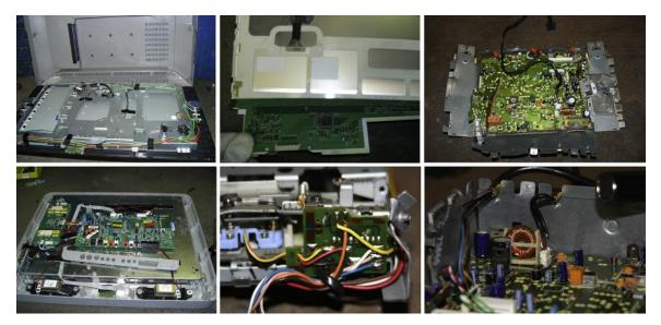
FIGURE 22.15 Different levels of material connections and material combinations (both physical and chemical) of printed wire boards in e-waste.
