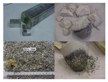
FIGURE 22.4 The effect of scrap surface area (left) on recovery (right) of two scrap types. Top: AlSi9 alloy and the flux/ metal after, which creates a clean melt and salt slag. Bottom: Melting recovery is held back by inactive alumina coating scrap, so scrap with a higher surface area/volume ratio has a lower recovery rate, creating under static melting conditions various droplets in slag (Xiao and Reuter, 2002).
