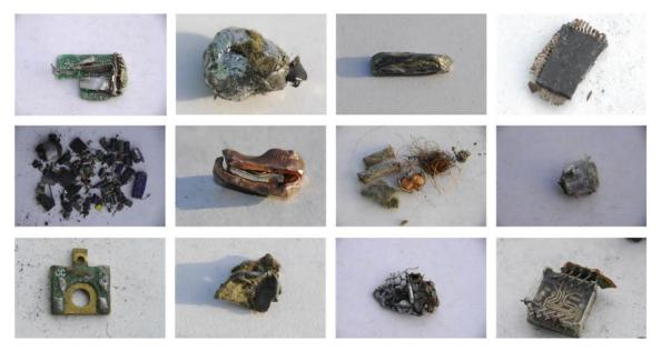
FIGURE 22.39 Particulate quality (determining recyclate quality and recovery/losses) as a function of design. An impression of unliberated and multimaterial particles as found in various WEEE recyclates.
