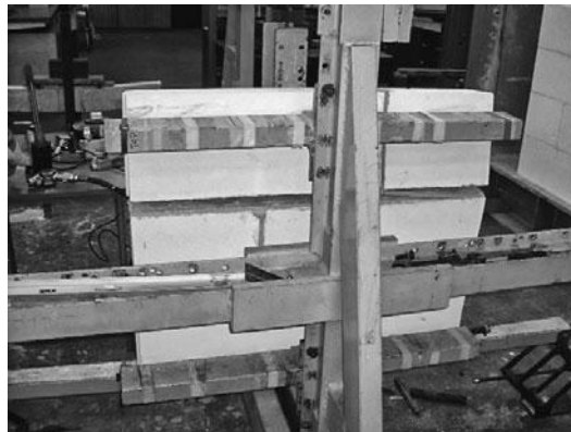
Figure 13.6 Failure of an aircrete wall using thin layer mortar under four-point loading
