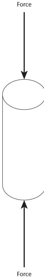
Figure 4.2 Schematic illustration of an object subjected to a compressive force or load
