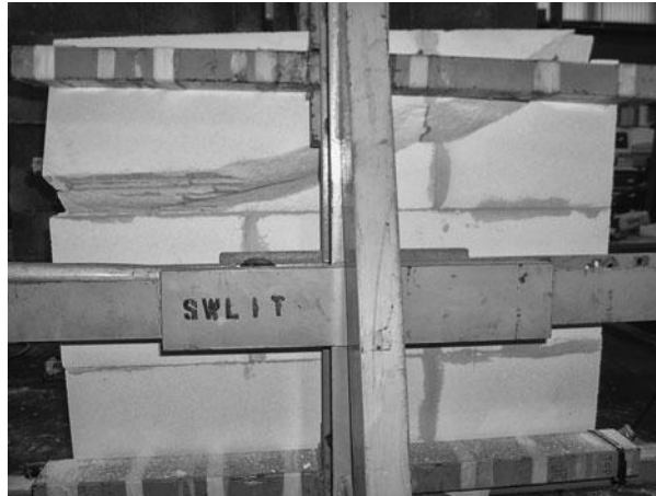
Figure 13.5 Failure of an aircrete wall using conventional mortar under four-point loading
