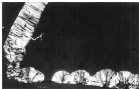
Fig. 7.21 Surface devitrification of a corroded and a newly formed \text{NaPO}_3 -glass surface. A glass rod was broken in vacuum immediately before the heat treatment. In this way, in addition to the corroded surface ( upper left corner ) a new surface was generated ( bottom part ). While at the newly formed surface only a few spherulites are detected, the corroded surface is covered by thousands of crystalline needles growing perpendicular to the surface
