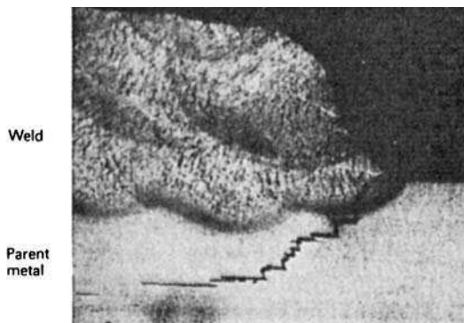
Fig. 11.12 Lamellar tearing near a weld (The Welding Institute).
