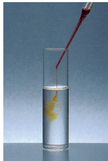
Addition of bromine to an alkene results in almost immediate loss of the red-brown color of \text{Br}_2 as the reaction takes place.
