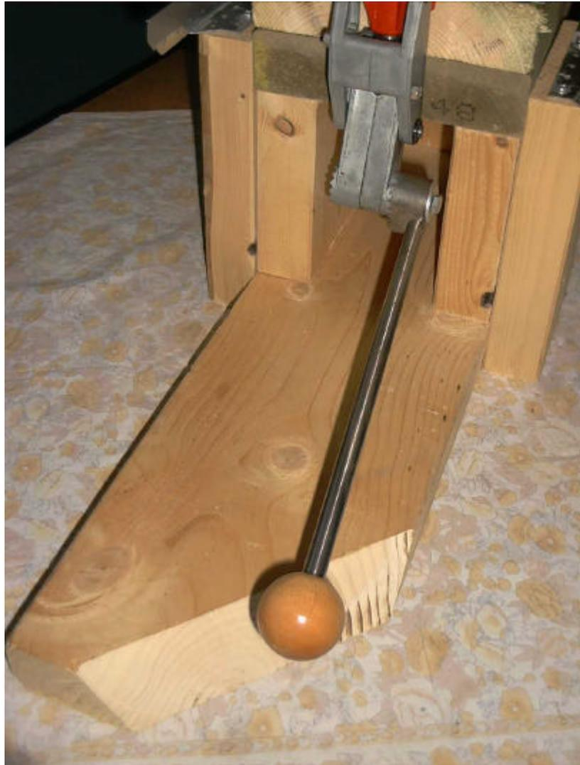
This quick and easy fix allowed us to work with the tabletop set-up with no problems at all, we was able to use a Lee Challenger, A Lee Turret and a Lee Pro 1000 with this set-up. As a special we set up Lee Challenger presses, and used Lee AutoMator kits to convert the press into a Lee Pro 1000 configuration.
