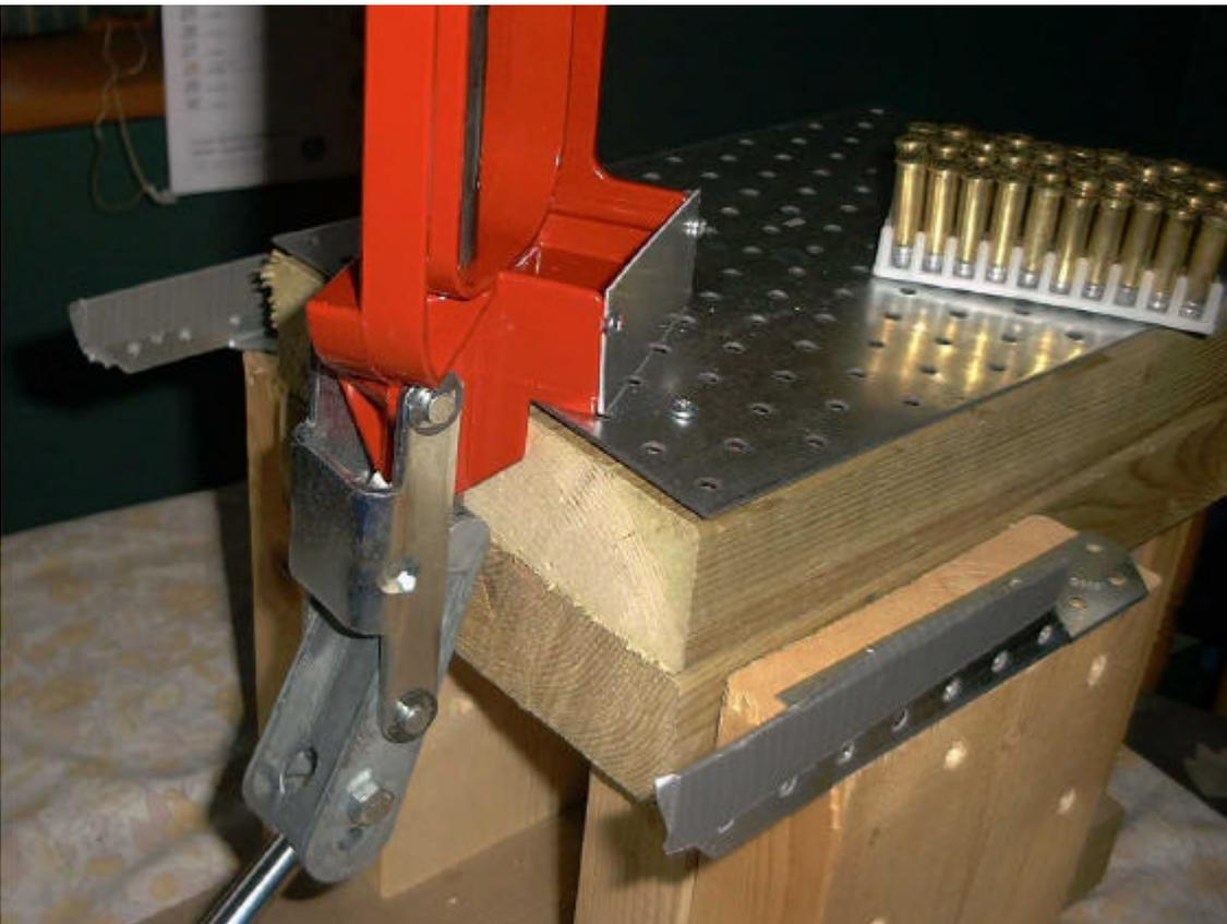
Details of the attachments and the exchangeable press mounts, the press fastens to the mount with 3 short 1/4" screws, the mount itself by 4 wood screws.
