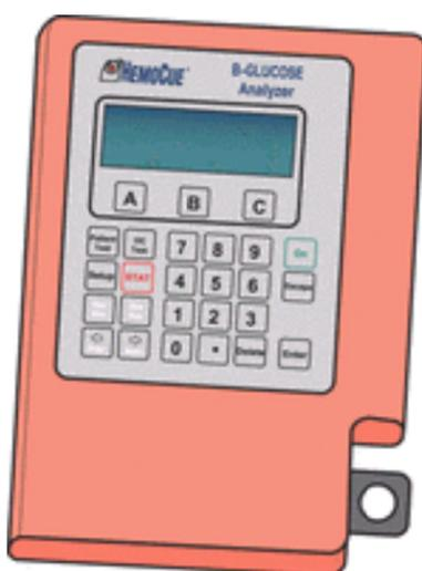
**FIGURE 6.2** Portable blood glucose analyzer (Source: HemoCue, Mission Viejo, California, USA.)
