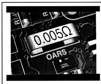
*IRC's OARS series Surface Mount sense resistor. As low as 5mΩ standard, rated at 1W with <30ppm/°C TCR. Mounting configuration minimizes TCR of copper leads*
