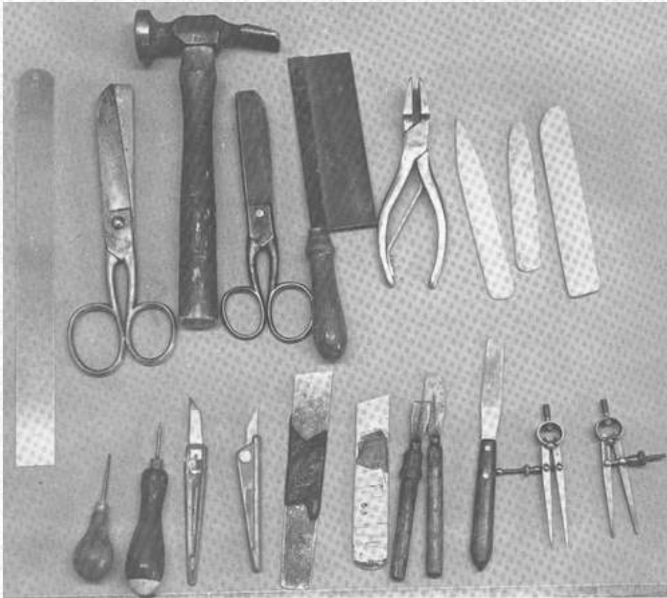
Figure 2 - Basic tool: top, left to right, metal foot rule, large shears, backing hammer, smaller shears, tenon saw, band nippers, three bone folders; bottom, left to right, two bradawls, two cutting knives, two paring knives, three palette lifting knives, two pairs of dividers.
