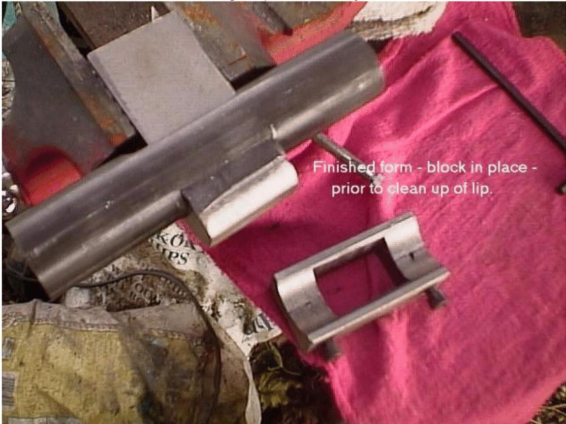
Just about ready to weld on the prepared mag well assembly now. Just need to dress down the lips.
