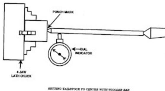
Make a light pass and check both ends to see if they measure the same. If not, adjust the tail stock and make another pass. Repeat the above operations until the bar measures the same on both ends.
