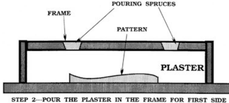
We must then heat the mold halves in an oven at or about 400 degrees F (this temperature may range from 300 to 1500 degrees F) to drive off all free water and convert the gypsum again to CASO. This may require twenty or more hours.
