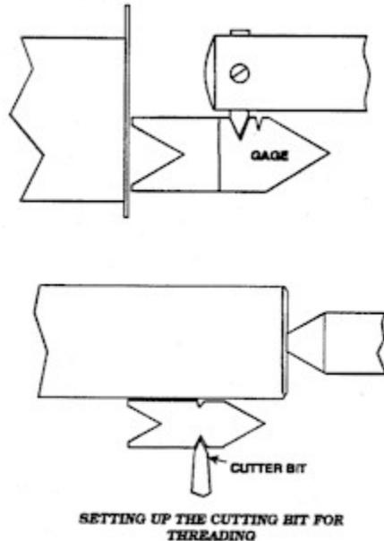
Start the first cut, close the half-nuts on the number “1” line of the dial and feed the tool with the compound until the tool just scratches a fine line, indicating the thread. Shut down the lathe and test this line with the thread-pitch gauge to see that the lathe is cutting correctly. The cross feed of the carriage must always be up tight to the cross-feed stop before moving the tool with the compound feed.
