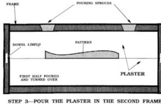
The pattern and the piece cost are much higher than for sand castings, but this cost is often justifiable because of the better finish and the elimination of machining. With these permeable plaster molds; eliminating the chemically combined water from the gypsum is not necessary, so drying requires less time.
