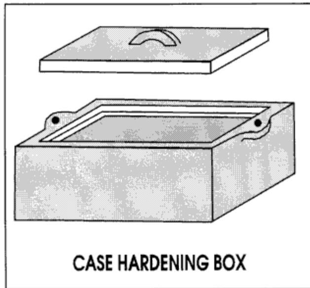
Most mild steels do not come with enough carbon to enable them to be hardened by heating and quenching, as are the higher-carbon-content tool steels. However, if carbon is added to the steel, it can be made to harden upon quenching. There are many methods of adding carbon. In the processes, the heated steel absorbs the carbon from the outside. The interior of the metal does not absorb the added carbon and so remains soft after quenching. A hard carbonous surface, or case, is formed on the metal.
