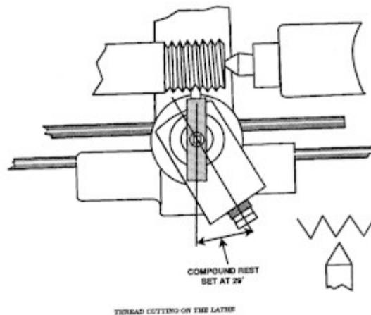
The compound slide is used to feed the tool into the work. By feeding the tool on the 60° angle to which the compound slide is set, the tool cuts on one side only, and it can be given a side rake to make the chip clear the thread groove. If the tool is fed in square with the work, it must cut on both sides. No side rake can be used, and the two opposing chips will interfere and jam in the cut.
