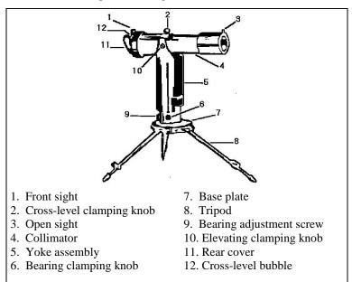
Figure G-1: Collimator M1A1
