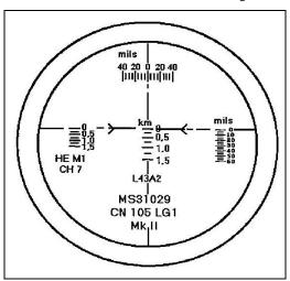
Direct Fire Telescope set to zero
