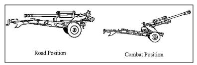
Figure 2-1: Gun Configurations
