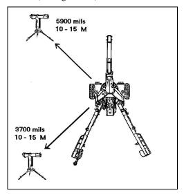
Figure G-2: Collimator Placement
