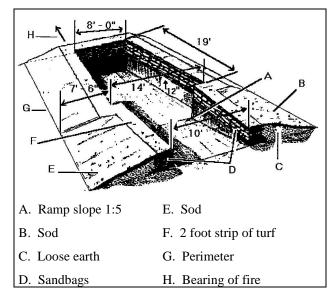
Figure B-1: Gun Pit Construction
