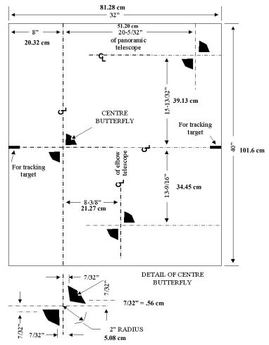
Figure 5-2: The Target Testing Sight
