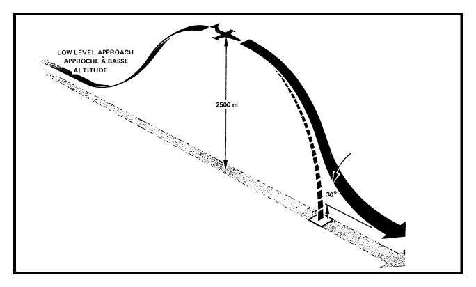
Figure 1-2-16 Rocket and Cannon Attack - 30 Degree Dive
