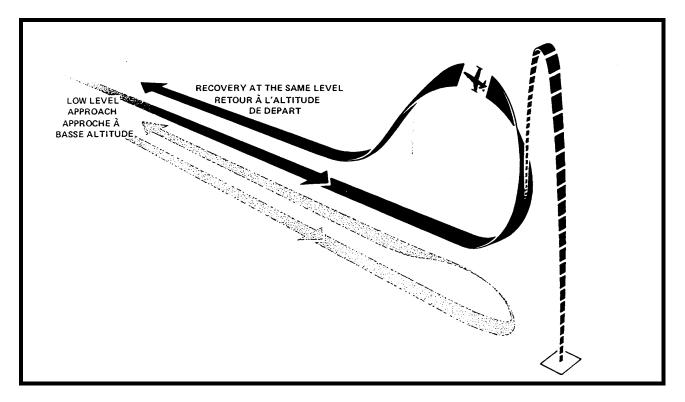
Figure 1-2-14 High Angle Toss Bombing
