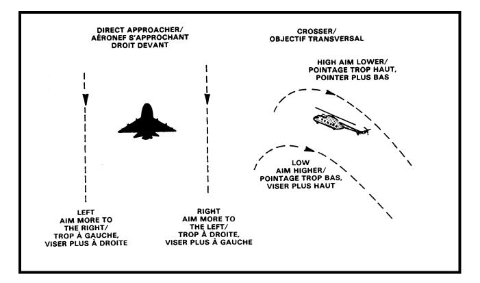
Figure D-3 Superimposing Tracer on the Target
