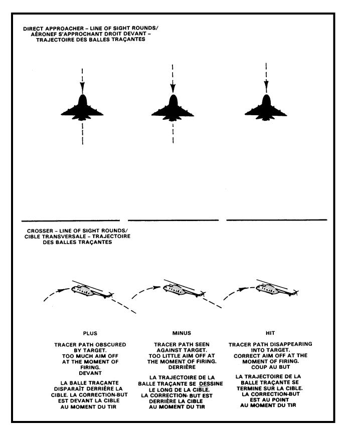
Figure D-4 Reading the Tracer and Correcting Aim-Off
