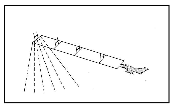
Figure 3-4-3 Point of Aim for Oblique High-speed Targets
