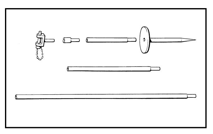
Figure A-5 The Ground Mount Disassembled
