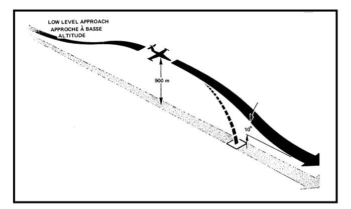
Figure 1-2-15 Rocket and Cannon Attack - 10 Degree Dive
