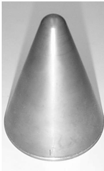
Figure 1. Standard 81mm shaped charge liner.
