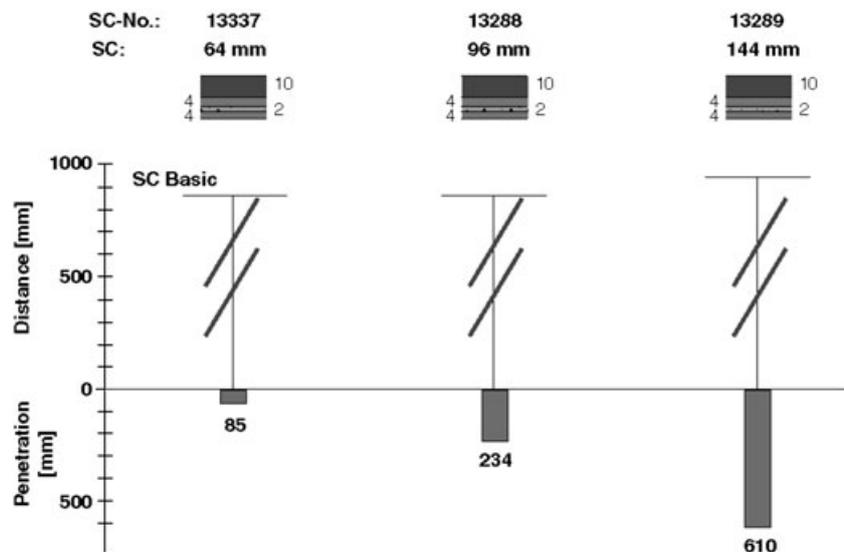
**Figure 8.** Residual penetration of shaped charges with different diameters against ERA 4/2/4.
