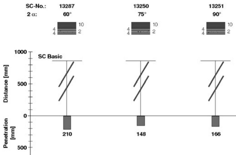
**Figure 2.** Layout of test setup with the achieved result of 3 liner angles of 60°, 75° and 90°.
