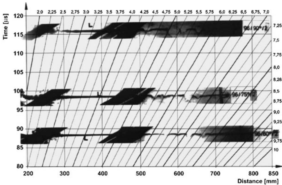
Figure 4. Disturbed jet after 4/2/4 ERA armor in the time distance plot.
