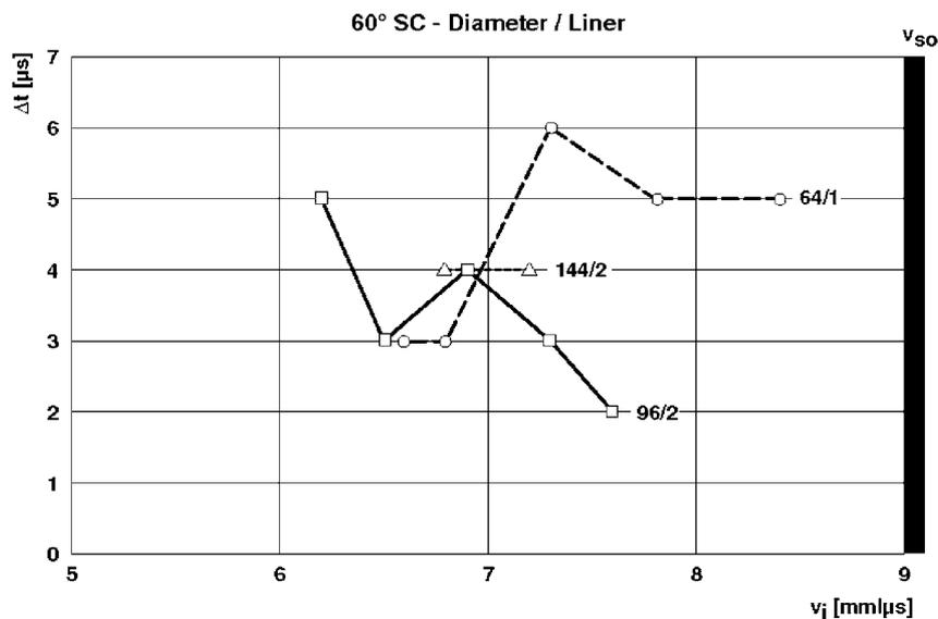
**Figure 14.** Time frequencies of disturbances of the jets of shaped charges with different diameters by the ERA sandwich 4/2/4
