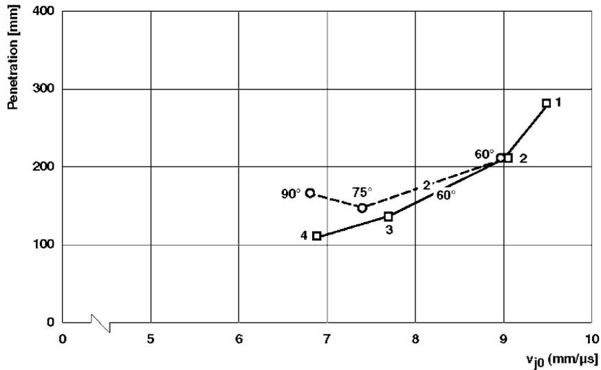
Figure 7. Residual penetration in mild steel after a 4/2/4 ERA sandwich as a function of jet tip velocity for different liner geometries – liner angle and liner thickness – of a 96 mm shaped charge.
