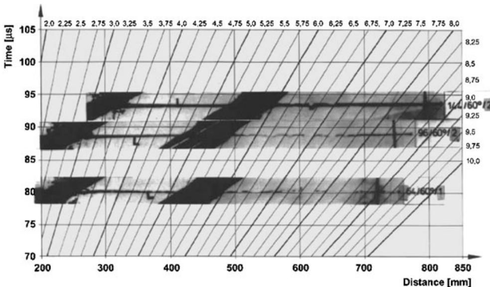
**Figure 10.** Flash X-ray pictures of the different charge sizes of 64 mm, 96 mm and 144 mm in the time distance plot after the 4/2/4 ERA sandwich.
