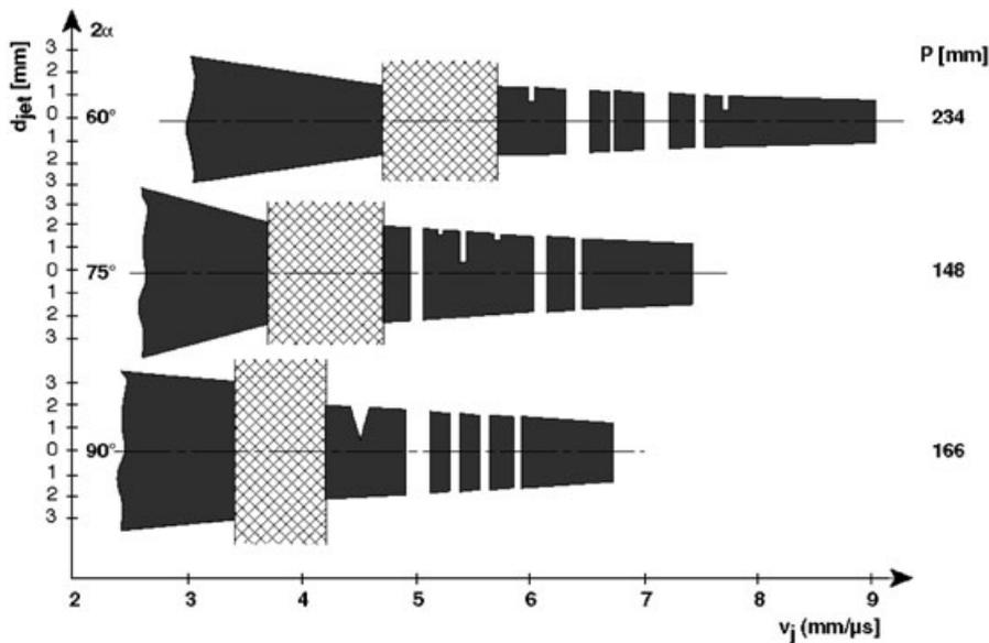
Figure 5. From the flash X-ray pictures analyzed jet diameters and disturbed jet regions as a function of jet velocity.
