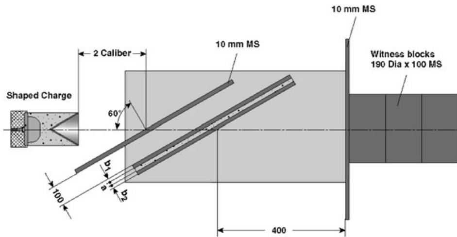
**Figure 1.** Test setup to measure the disturbances of the shaped charge jets by flash X-ray and to get the residual penetrations.
