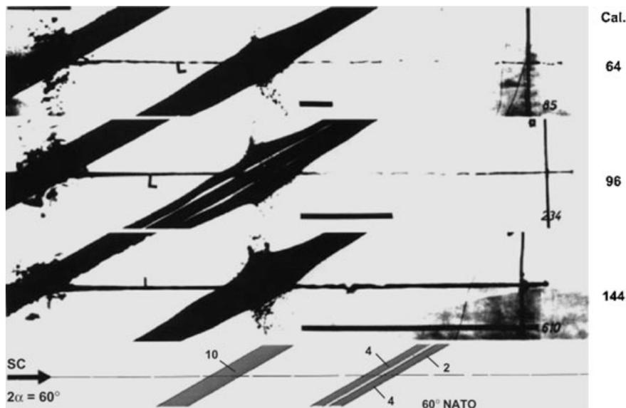
**Figure 9.** Flash X-ray pictures of the jets before and after the 4/2/4 ERA target from shaped charges of 64 mm, 96 mm, 144 mm base diameter; the target setup is sketched at the bottom.
