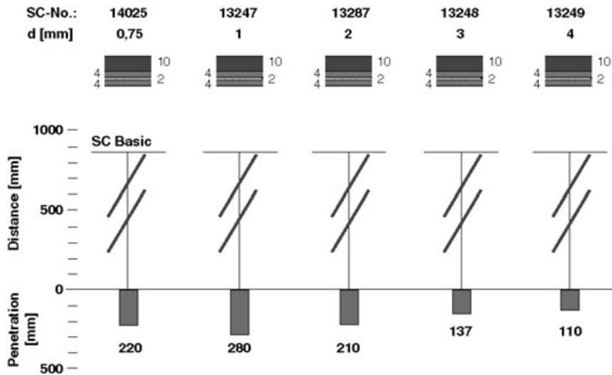
Figure 6. Test results of the different liner wall thicknesses against light ERA target.
