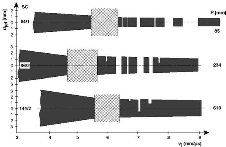
**Figure 11.** Analyzed jet diameters and disturbances of the analyzed flash X-ray pictures of the 3 fired shaped charge diameters of 64 mm, 96 mm and 144 mm.
