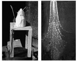
Figure 11. Selectable mode warhead test stand (left). X-ray of case 1 fan jet at 80 microseconds (right).
