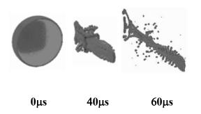
Figure 6. Final CTH model of the dual detonator hemispherical liner.
