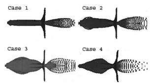
Figure 10. Jet profile as a function of detonator location at 35 microseconds.
