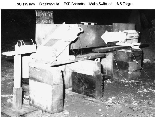
Figure 3. Test setup with the covered glass target under  $55^\circ$ .
