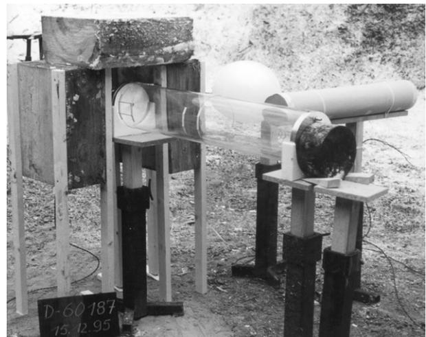
**Figure 3.** Picture of test setup with the cavity charge on the left side, the plexiglass tube, which can be evacuated and the argon bombs in the background.
